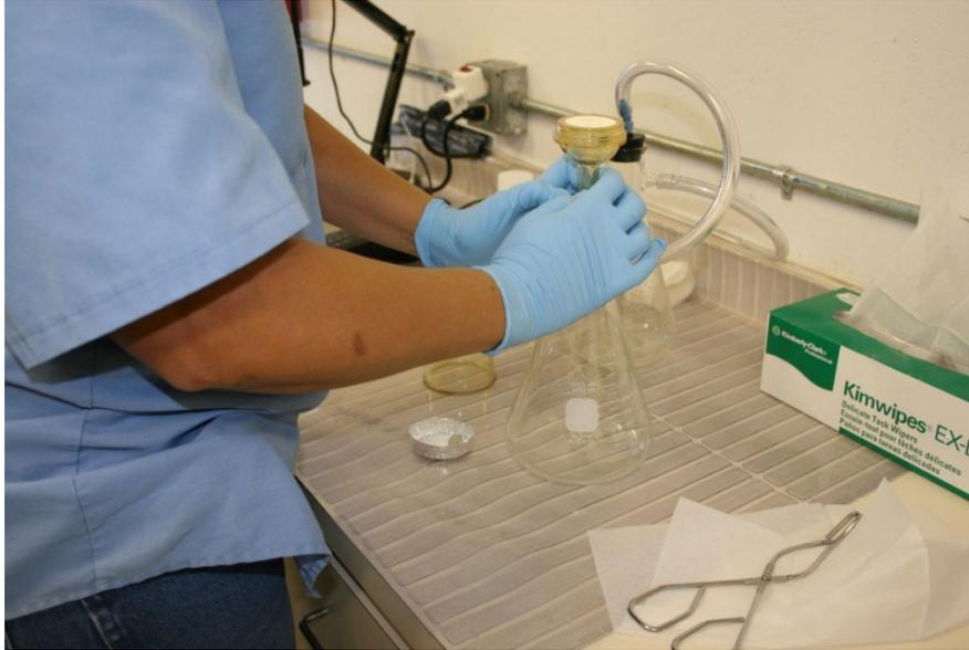
**Total dissolved solids** - The weight per unit volume of all volatile and non-volatile solids dissolved in a water or wastewater after a sample has been filtered to remove colloidal and suspended solids. The lab tech is filtering a wastewater sample.
