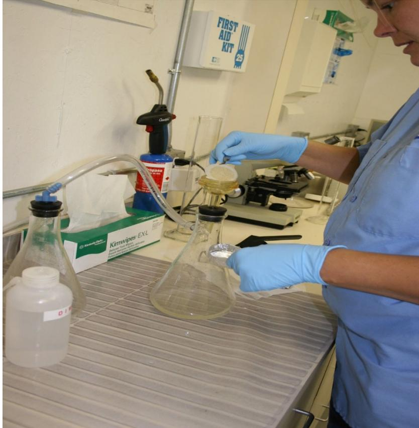
Lab tech removing filter for TSS analysis.
