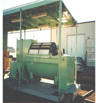
The biological growth that becomes attached to the media assimilates the organic materials in the wastewater. Aeration is provided by the rotating action, which exposes the media to the air after contacting them with the wastewater. The degree of wastewater treatment is related to the amount of media surface area and the quality and volume of the inflowing wastewater.
