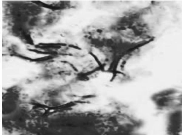
Figure 7. An typical view of Microthrix parvicella (gram stain x 1000) after extended PAX treatment.
