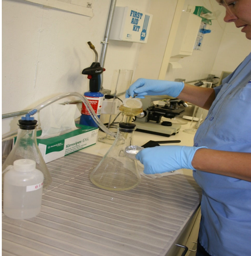
Lab tech removing filter for TSS analysis.
