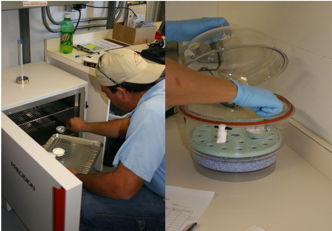
Top left, filters being baked at 105°C. Right photograph, filters in desiccant.
