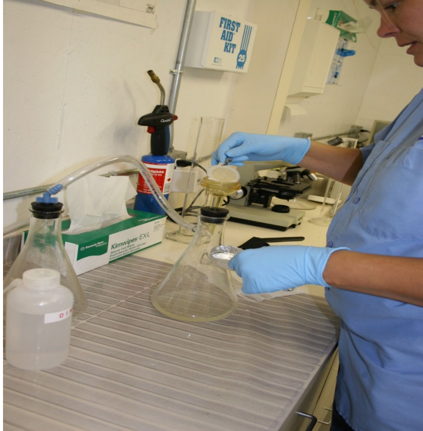
Lab tech removing filter for TSS analysis.
