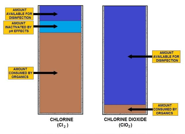
THE DIFFERENCE IN USING CHLORINE AND CHLORINE DIOXIDE AS A DISINFECTANT
