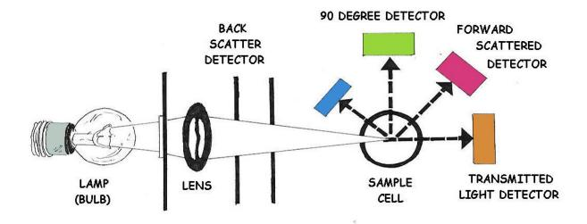
HOW AN TURBIDIMETER WORKS
