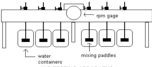
JAR TESTING APPARATUS
