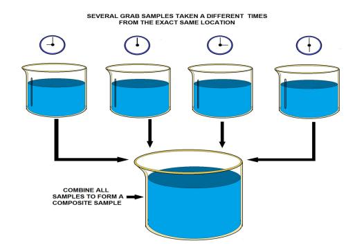
MAKING A COMPOSITE SAMPLE FROM GRAB SAMPLES DIAGRAM
