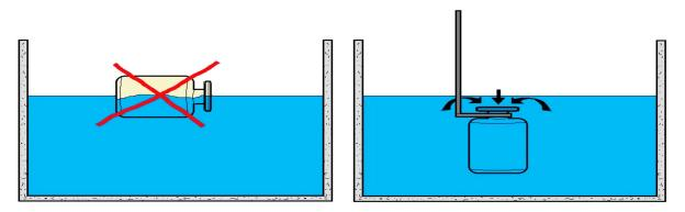
PROPER MATHOD OF TAKING IMMERSE TYPE WATER SAMPLES.
