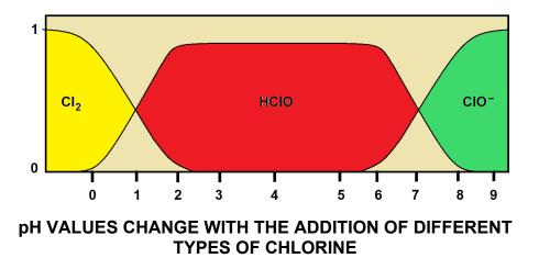
Mathematically, pH is the measurement of hydroxyl ion (H+) activity and expressed as the negative logarithm of the activity of the (solvated) hydronium ion, more often expressed as the measure of the hydronium ion concentration.
