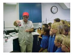
As the iron and manganese begin to oxidize, the sample will turn varying shades of brown, indicating the presence of oxidized iron and or manganese. Samples which retain a brown or yellow color indicate that the oxidation process is incomplete and will require a higher dosage of  $KMnO_4$ .
