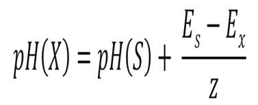
The difference between the two measured emf values is proportional to pH. This method of calibration avoids the need to know the standard electrode potential. The proportionality
