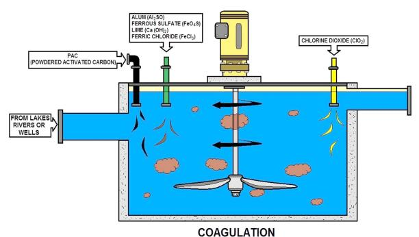
(FLASH MIXING / WATER IS AGITATED TO EVENLY BLEND COAGULANTS AS FAST AS POSSIBLE)
