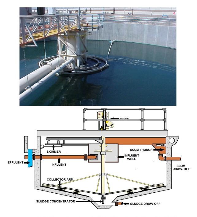
CIRCULAR CLARIFIER AND COLLECTOR MECHANISM
