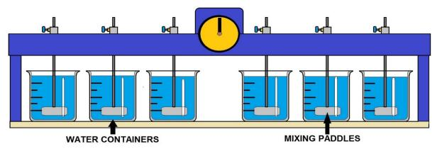
FLOCCULATION / COAGULATION JAR TEST UNIT
