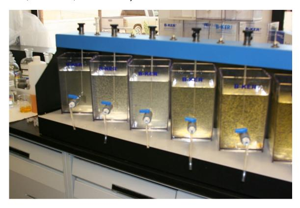
Jar Testing –Coagulation and Flocculation at different doses and conditions
