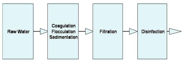
Suspended particles carry an electrical charge which causes them to repel one another. The conventional process uses alum (aluminum sulfate or ferric chloride) and cationic polymer to neutralize the charge. That allows suspended particles to clump together to form more easily filtered particles.
