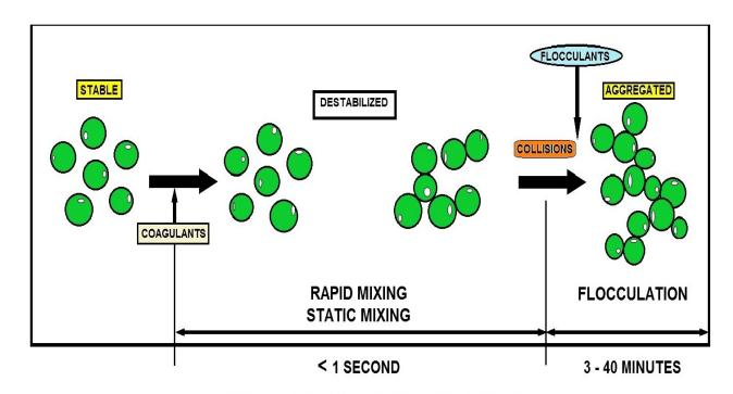
BASIC COAGULATION AND FLOCCULATION DIAGRAM #2
