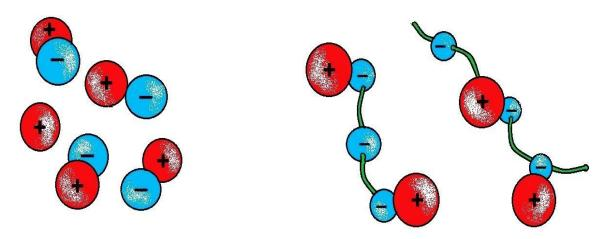
COAGULATION VS FLOCCULATION MOLECULAR LEVEL DIAGRAM
