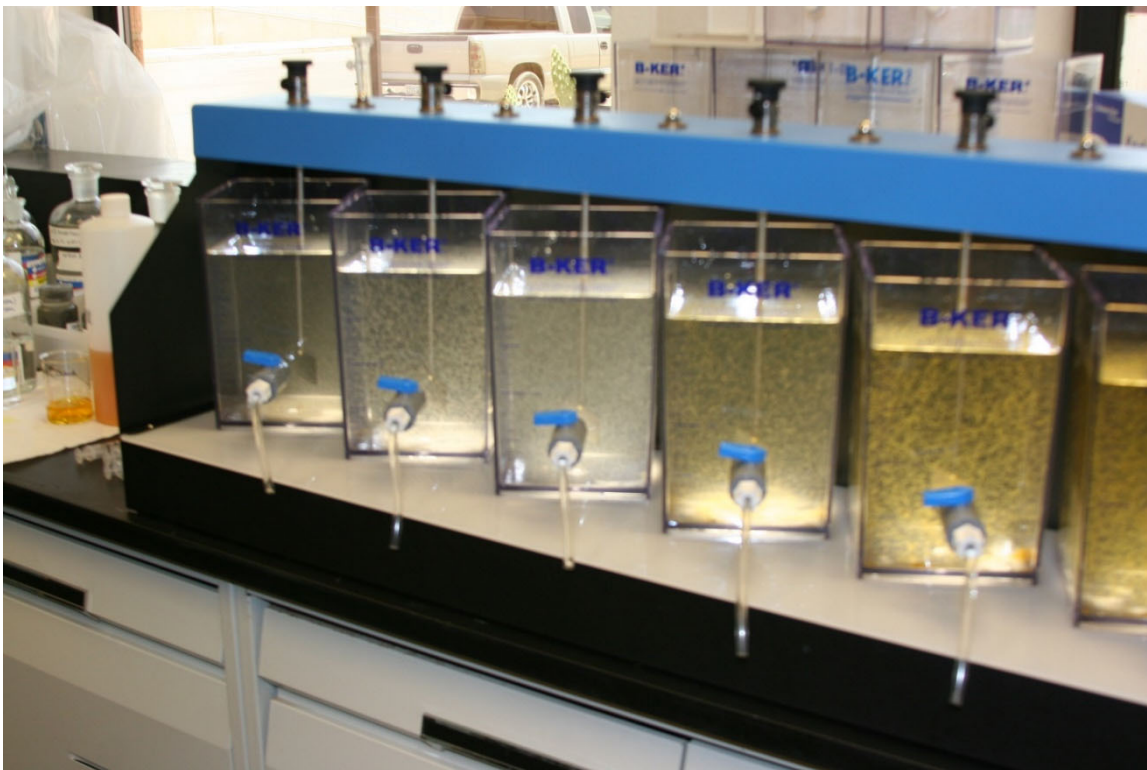
Jar Testing –Coagulation and Flocculation at different doses and conditions
