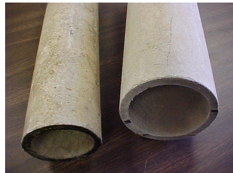
ACP Pipe with illegal power saw cut marks.
