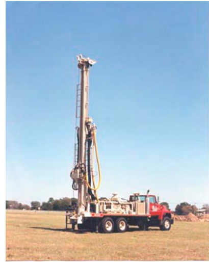
Typical Rotary Rig
