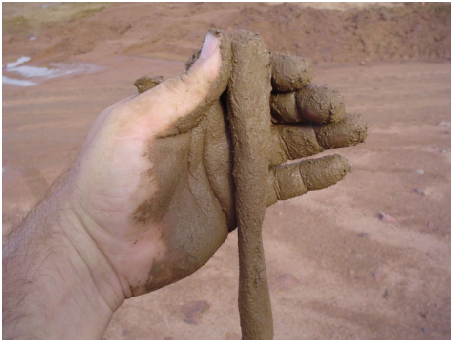
Ribbon Soil Test
