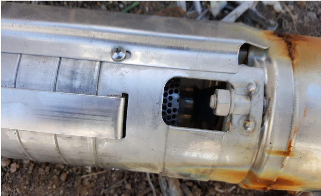
Pump and motor connection.
