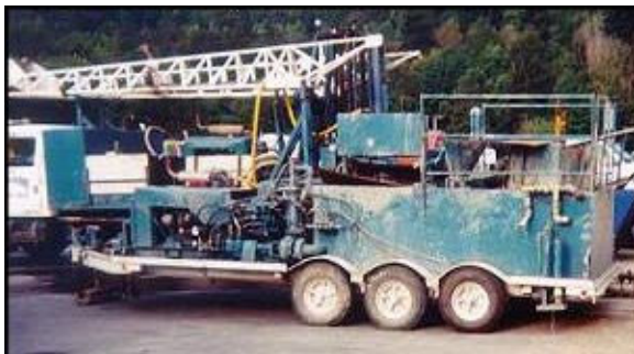
Small Self-Contained Mud System
