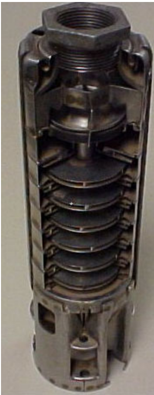
Left- Cut away of a small turbine pump without the motor.
