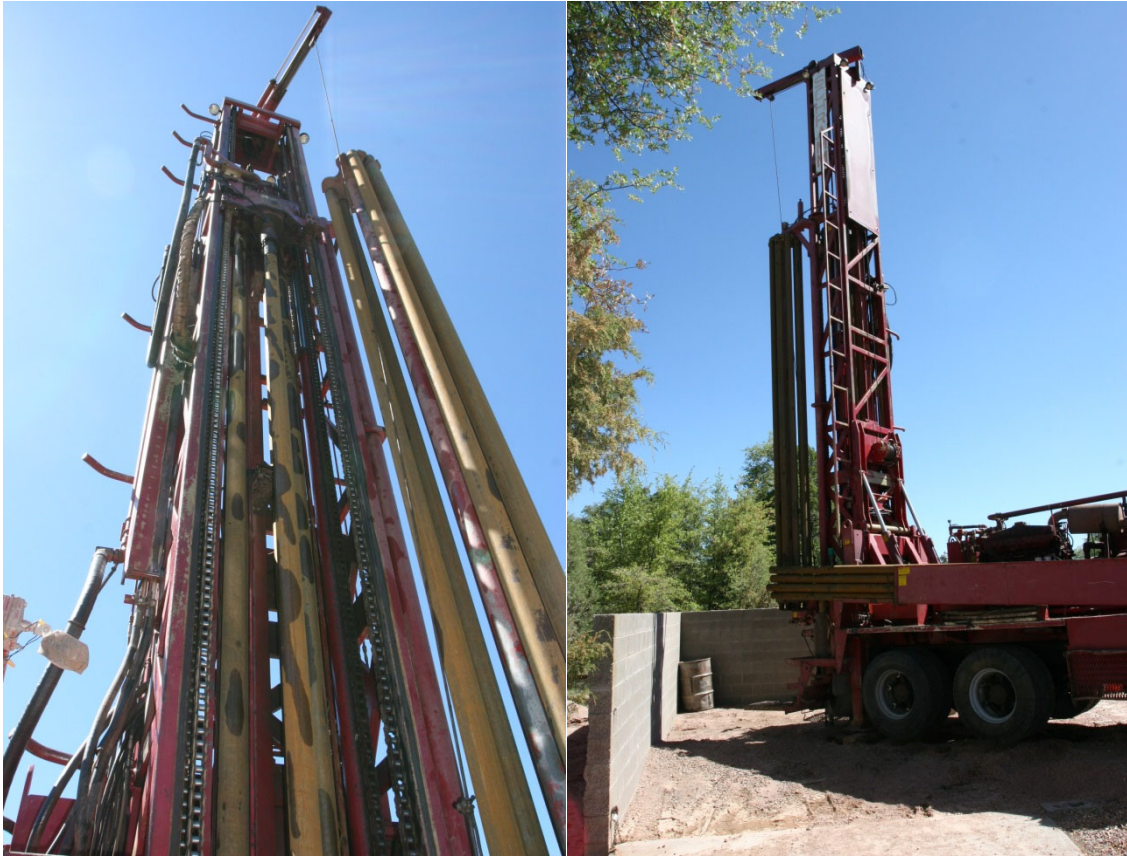
Top, drill rigging mast. Below, drilling rods on carousel and rack, notice copper pipe thread coating which prevents thread lock during high torque.
