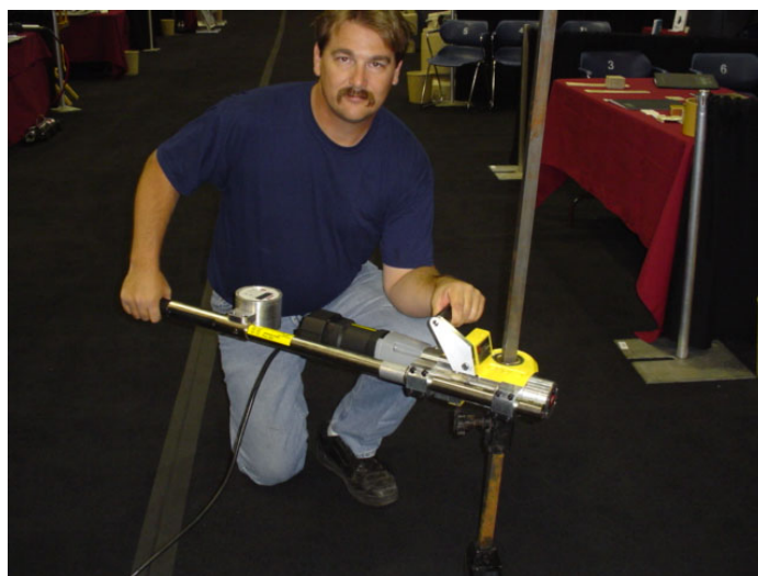
Portable valve exercising machine.
