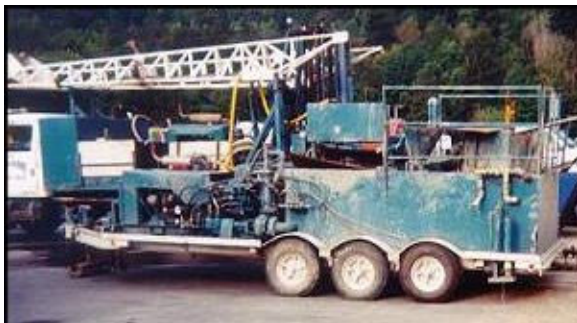
Small Self-Contained Mud System
