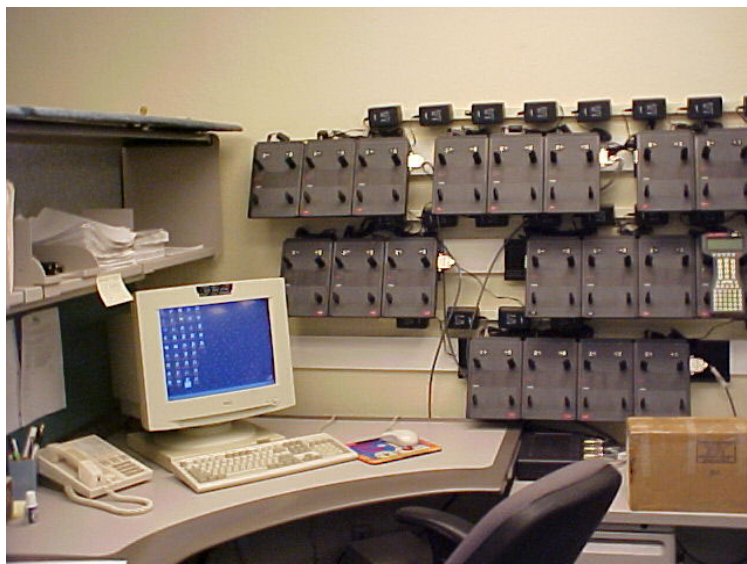
Computerized handheld electronic meter reader “station”
