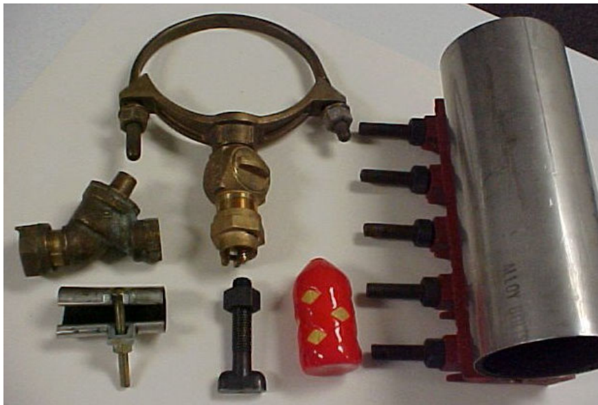
Common distribution fittings. Single check, Poly Pig, 1- inch repair clamp, 4-inch full circle clamp, T- Bolt and a corp. and bronze saddle.
