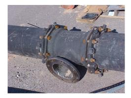
Notice the type of pipe connection device, it is known as a "Restraining Flange".
