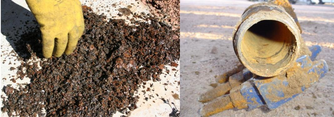
Rust and debris from cleaning a steel main.
