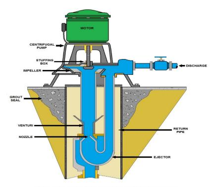
VERTICAL TURBINE INSTALLATION DIAGRAM
