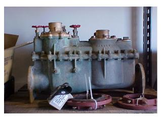
**Meter Purpose**: Is to properly record the flow of water in a part of the distribution system. To properly account and bring revenue to the City or Water Provider.
