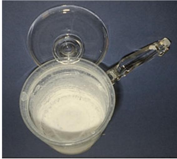
When hard water is heated, scale forms much faster. In particular, when the magnesium hardness is more than about 40 mg/l (as  $\text{CaCO}_3$ ), magnesium hydroxide scale will deposit in hot water heaters that are operated at normal temperatures of 140-150°F (60-66°C).
