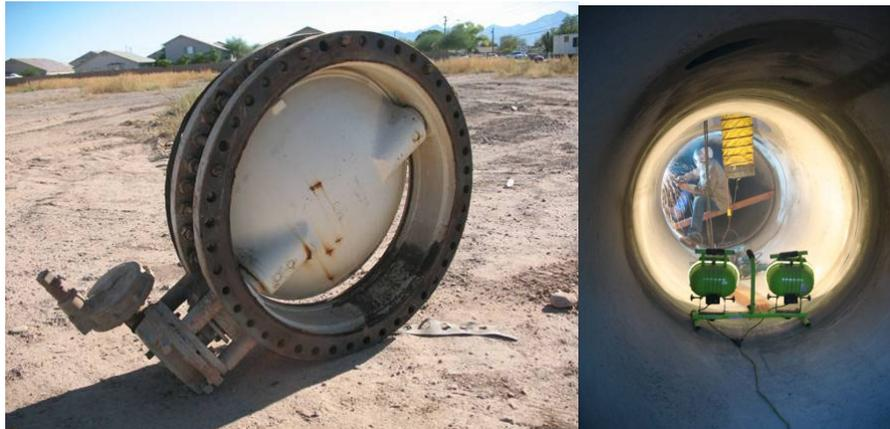
A broken 54-inch Butterfly and a worker inside the water main preparing the interior surface. Notice, this is a Permit Required Confined Space. Hot work permit is also required. Side note, there is a plastic version of the 54 and 60-inch butterfly valve.
