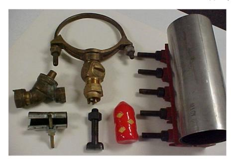
Common distribution fittings. Single check, Poly Pig, 1- inch repair clamp, 4-inch full circle clamp, T- Bolt and a corp. and bronze saddle.
