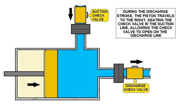
PISTON TYPE -POSITIVE DISPLACEMENT PUMP
