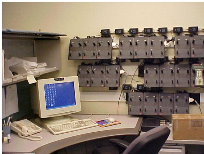
Computerized handheld electronic meter reader “station”
