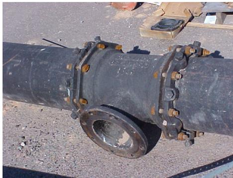
Notice the type of pipe connection device, it is known as a "Restraining Flange".
