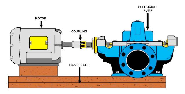
FLEXIBLE COUPLED PUMP AND MOTOR
