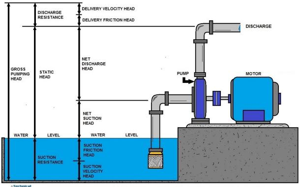
**FACTORS IN DETERMINING A TYPICAL PUMP INSTALLATION**
