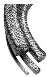
When replacing packing, be sure the packing fits uniformly around the stuffing box. If you have to flatten the packing with a hammer to make it fit, **YOU ARE NOT USING THE RIGHT SIZE.** Pack the box loosely, and set up the packing gland lightly. Allow a liberal leak-off for stuffing boxes that operate above atmospheric pressure.
