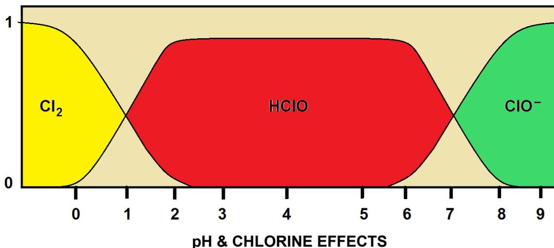
Chlorine present as Cl, HOCl, and OCl<sup>-</sup> is called *free available chlorine* and that which is bound but still effective is *combined chlorine*. A particularly important group of compounds with combined chlorine is the chloramines formed by reactions with ammonia.
