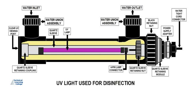
Ultraviolet light for disinfection was primarily used in the wastewater industry because of its effectiveness to deactivate microorganisms and not having to dechlorinate the effluent for discharge. In drinking water, UV has become popular because it does not produce trihalomethanes, but there is no residual disinfectant. Another consideration is the cost to operate and maintain the UV unit, which is generally higher than simple chlorination.
