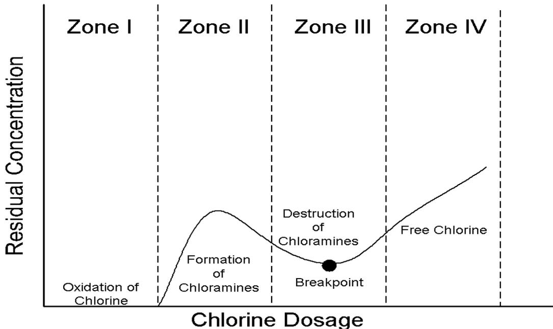
The graph shown on the last page depicts the chlorine residual as a function of increasing chlorine dosage with descriptions of each zone given below (Drawing by Erik Johnston, adapted from Reynolds and Richards, 1996).
