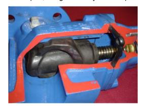
It is suggested to listen to the Valve Key when shutting down a Gate valve. You will easily hear it sing as you shut the water off or leak by. It is very easy to create a water hammer with opening or closing a Gate valve. Always take your time when operating a gate valve or any valve. I know that most of you will not listen to me and you will end up breaking plastic water services and customer's water lines at first.
