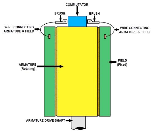
DIAGRAM SHOWING MECHANICAL CONSTRUCTION
