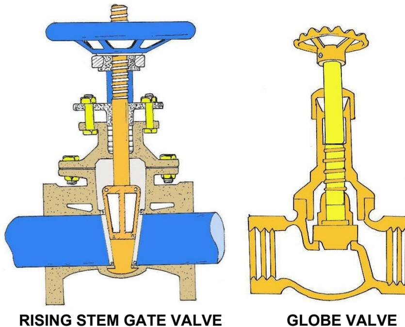
The valve should be welded onto the line with the disc in the fully closed position. Leaving it even partially open can cause distortion and leaking. Allow time for the weld to cool before operating the valve the first time in the pipeline.
