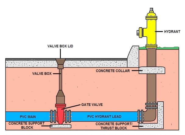
PROPER FIRE HYDRANT AND ISOLATING GATE VALVE INSTALLATION
