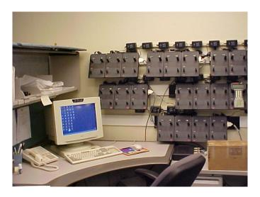
Computerized handheld electronic meter reader "station"
