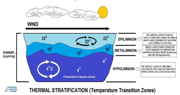
Thermal stratification is possible as **water becomes less dense when heated**, meaning water weighs less per unit volume. Therefore, warmer water will be lighter and colder water will be heavier. Due to this, there will always be a level of "self-induced" thermal stratification in a water storage.
