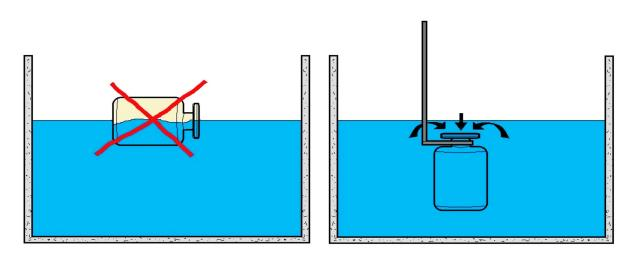
PROPER MATHOD OF TAKING IMMERSE TYPE WATER SAMPLES.
