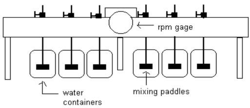
JAR TESTING APPARATUS
