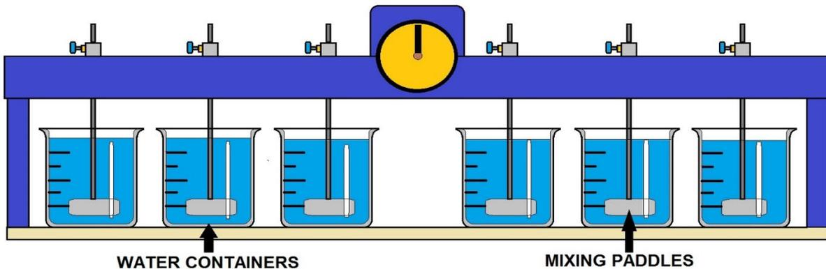
**FLOCCULATION / COAGULATION JAR TEST UNIT**
