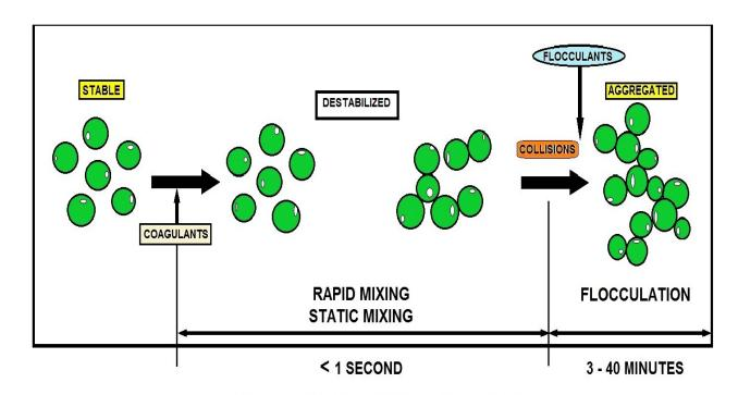
BASIC COAGULATION AND FLOCCULATION DIAGRAM #2
