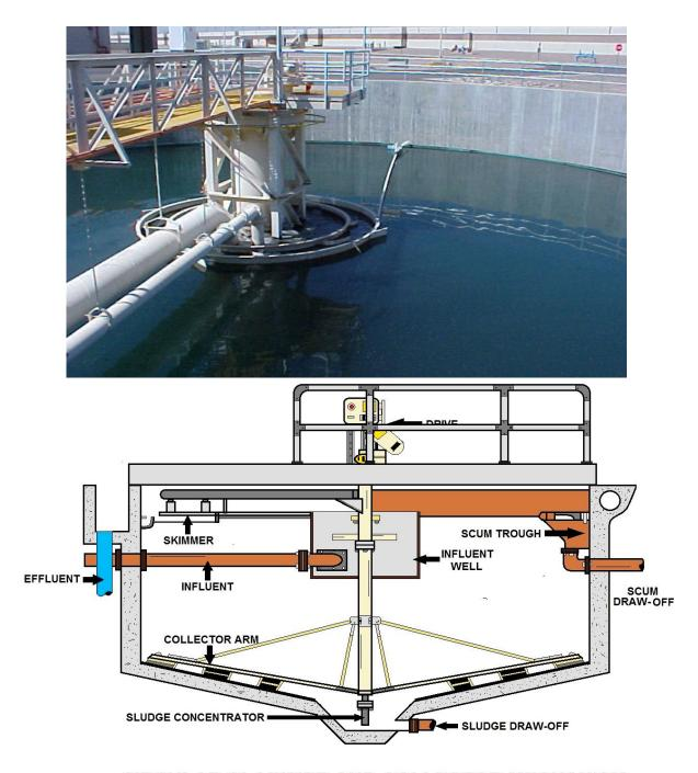
CIRCULAR CLARIFIER AND COLLECTOR MECHANISM
