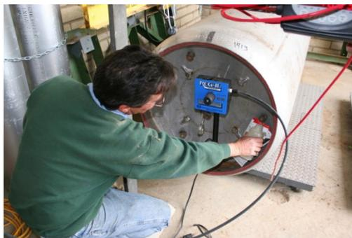
Here is an operator checking for  $\text{Cl}_2$  leaks with Ammonia. If there is a  $\text{Cl}_2$  leak, you will be able to see a white smoke. Even if you cannot smell the chlorine, the ammonia will find the leak.
