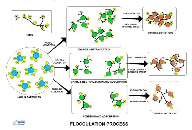
**Chemical Coagulation** in the water/wastewater treatment is the process of bringing suspended matter in untreated water together for the purpose of settling and for the preparation of the water for filtration.
