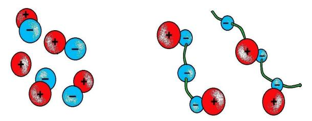
COAGULATION VS FLOCCULATION MOLECULAR LEVEL DIAGRAM
