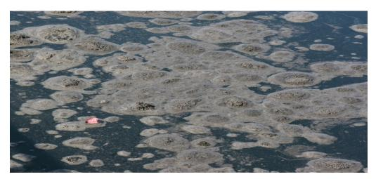
The above photo shows clumps formed by Powder Activated Carbon.
