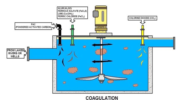
(FLASH MIXING / WATER IS AGITATED TO EVENLY BLEND COAGULANTS AS FAST AS POSSIBLE)
