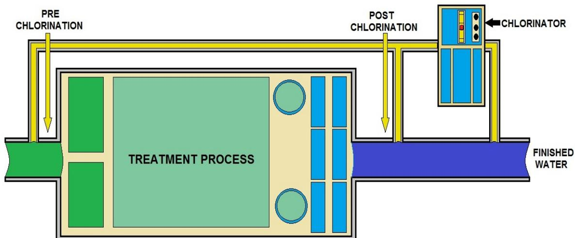
**CHLORINE FLOW IN A TREATMENT PLANT**
