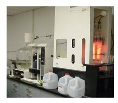
The principal problem with a distiller is that a small unit can produce only 2-3 gal (7.5 -11 Lt) a day, and that the power cost for operation will be substantially higher than the operating cost of other types of treatment devices.
