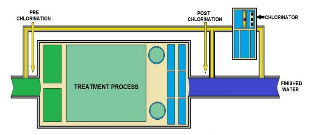
CHLORINE FLOW IN A TREATMENT PLANT
