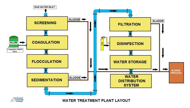
The design of a water treatment plant is determined by the water quality characteristics. Conventional water treatment plants include the steps as shown above if the quality of the source water is variable or poor. Direct filtration plants do not require sedimentation because the water quality characteristics are better.
