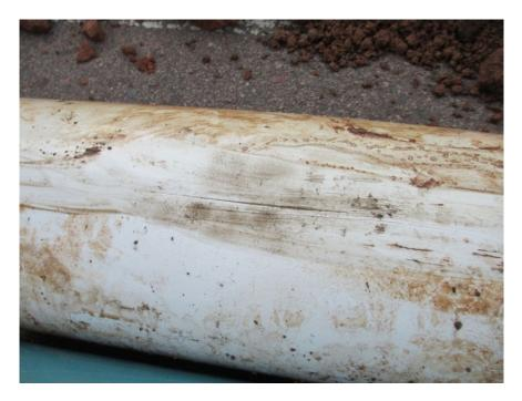
Generally speaking, water main breaks are much more intense that service leaks. This scenario with examine a hairline crack caused by poor installation. The water main was laid on a sharp rock without proper bedding. A slight water main leak is often confused with a service line leak and can be difficult to find.
