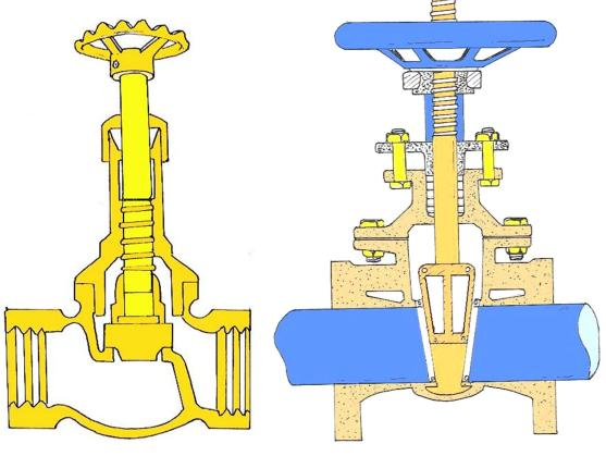
GLOBE VALVE VS RISTING STEM GATE VALVE
