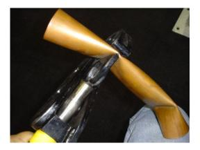
Copper Tubing Crimpers. Great if you are unable to get a shut-down. Just place this dude on the pipe. The problem is to fix that crimp when you are finished with the leak. They need to invent an uncrimper.
