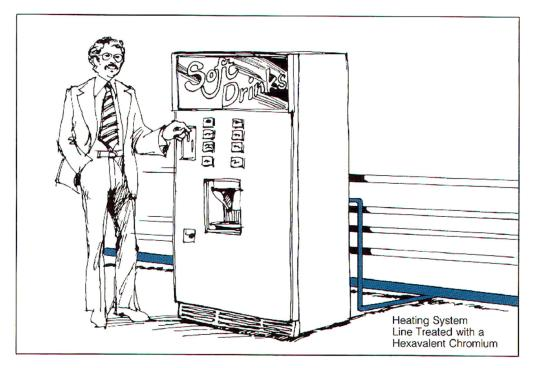
Several cross-connection have been made to soda machines, the one to worry about is when you have a copper water line hooked to  $CO_2$  without a backflow preventer.
