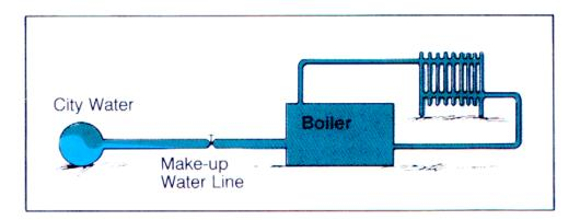
Example of backpressure being caused by heat.
