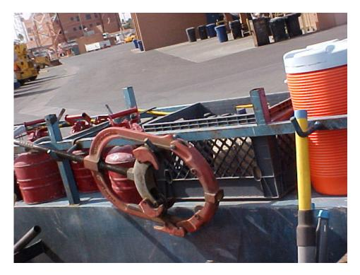
Here is a four-way pipe cutting tool used for iron pipe. Be careful not to break the wheels by over-tightening. I personally like 4-Ways because of the nice cut. You will learn to recognize the distinct snap of cut pipe. The only drawback to these cutters is cutting a small section out of the main.
