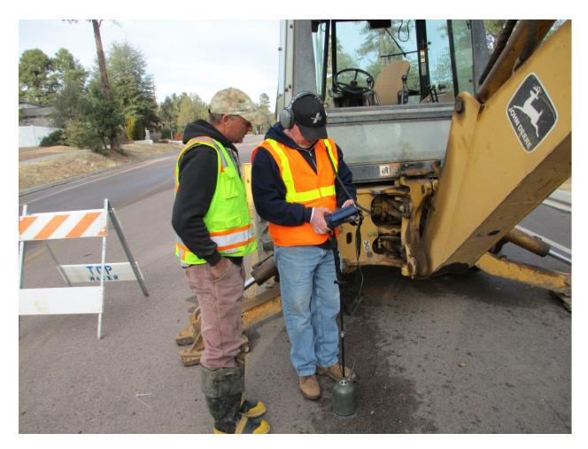
In this photograph, we see two men checking the results of a hydrophone. In areas of thick blacktop, it is difficult to locate small service leaks and slow water main breaks. A hydrophone is a microphone designed to be used underwater for recording or listening to underwater sound.
