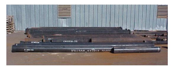
**Ductile pipe cement-lined iron pipe.** I've seen thousands of dollars of pipe that is dropped or moved with the front bucket of a backhoe and destroyed. This destroys the interior protection of the pipe, causing leaks which will start within in a short period of time, just a few years. I know that some of you welcome this as job security. Always protect and store all types of pipe covered and in a pipe rack. This goes for the proper storage of rubbers as well.
