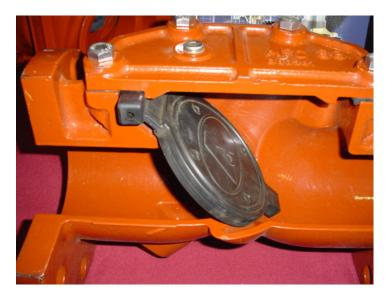
A beautiful swing check valve. Swing checks need to be maintained. I hate finding a swing check that is both buried and forgotten, rusted in place or, my favorite, the check was removed.
