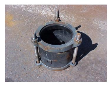
**Flex Coupling**--sometimes referred to as a Dayton; used to join pipes or to "cut-in a valve." You will learn that you can use different sizes to join pipe or even file out the inside diameter to adjust to larger pipes like ACP. This flex coupling only has three bolts. I like four or more for work with larger pipe work.
