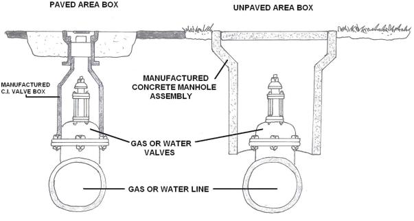
**TYPICAL VALVE BOX INSTALLATION DETAIL**
