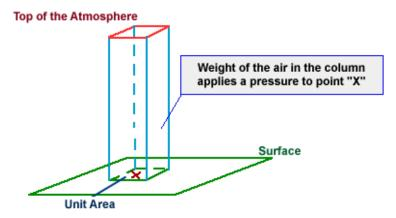
It is impossible to make a pressure measurement on the earth's surface unless it is made relative to atmospheric pressure. Therefore, a reference can be established at the atmospheric pressure level.
