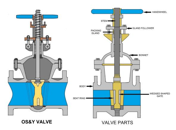
**OS&Y VALVE AND INTERNAL DIAGRAM**
