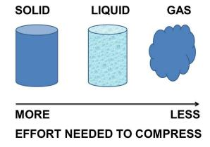
substances are compressed. Liquids already have their atoms close together, so they are hard to compress. Many shock absorbers in cars compress liquids in tubes.
