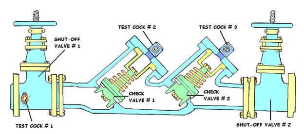
**DOUBLE - CHECK BACKFLOW ASSEMBLY DIAGRAM**
