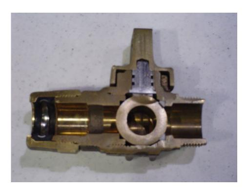
Above, a cut away of a brass Ball valve. Below a PRV.
