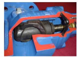
Therefore, there is little pressure drop or flow restriction through the valve. Gate valves are not suitable for throttling purposes. The control of flow is difficult because of the valve's design, and the flow of fluid slapping against a partially open gate can cause extensive damage to the valve. Except as specifically authorized, gate valves should not be used for throttling.
