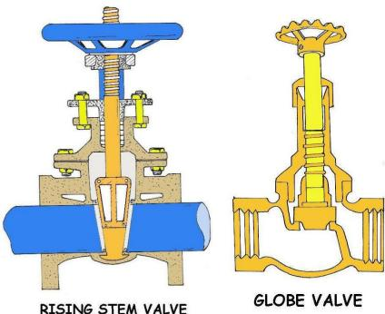
The valve should be welded onto the line with the disc in the fully closed position. Leaving it even partially open can cause distortion and leaking. Allow time for the weld to cool before operating the valve the first time in the pipeline. The preferred orientation of a globe valve is upright. The valve may be installed in other orientations, but any deviation from vertical is a compromise. Installation upside down is not recommended because it can cause dirt to accumulate in the bonnet.
