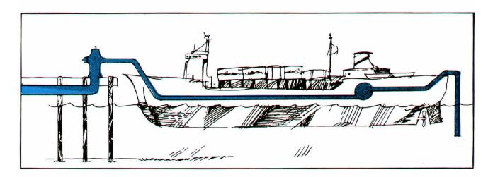
Here we see the backpressure of salt water back into the public water system from a ship's pressure pump. Most water providers are now requiring a RP assembly at the hydrant.
