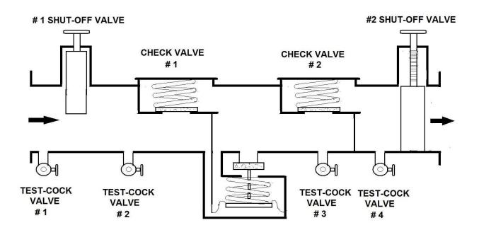
REDUCED PRESSURE PRINCIPLE BACKFLOW ASSEMBLY
