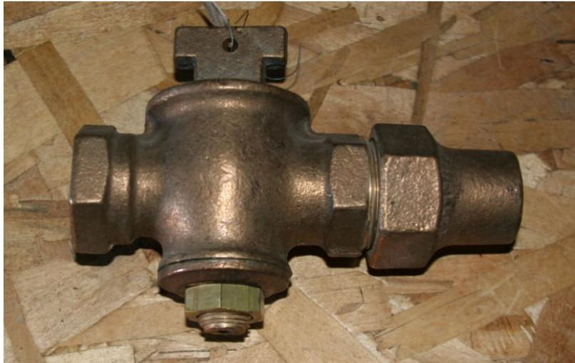
A Ball Stop with a flare fitting. It is difficult to find and even harder to find a person that knows how to flare copper pipe correctly. This may be one the finest copper fitting connection of all time, even stronger than sweating.
