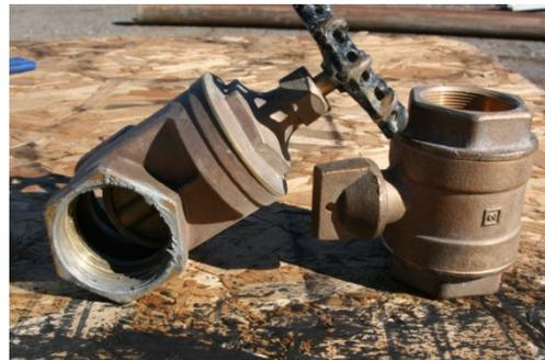
Brass or zinc is common for body, brass or iron for stem, brass or iron for ball, aluminum, stainless steel, or iron for handle including a Teflon seal in the ball housing. Flush the pipeline before installing the valve.
