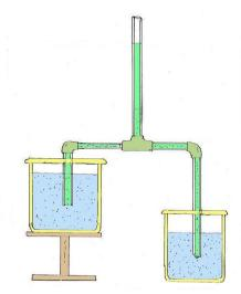
A siphon can be made by filling the tube, closing the ends, and then putting the ends under the surface on both sides. Alternatively, the tube can be placed in one fluid and filled by sucking on it. When it is full, the other end is put in place. The analysis of the siphon is easy, and should be obvious. The pressure rises or falls as described by the barometric equation through the siphon tube.
