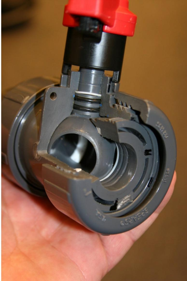
A cut away of a ball valve. The ball is made of plastic in this valve. The balls are not perfectly round but are egg shaped or elongated to make a good seal.
