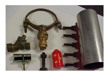
Common distribution fittings: Single check, Poly Pig, 1-inch repair clamp,4-inch full circle clamp, T- Bolt and a corp. and saddle. Note from Dr. Rusty, Single checks are not a backflow assembly and will probably stick open over time. I know that most systems will pay for these but unless you replace or test these checks, they will not hold up. Most fitting salesmen will not tell you this little tidbit. Notice the Corp, it is a ball type valve.
