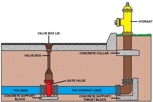
PROPER FIRE HYDRANT AND ISOLATING GATE VALVE INSTALLATION
