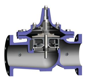
When no pressure is in the valve, the spring and the weight of the diaphragm assembly hold the valve closed.
