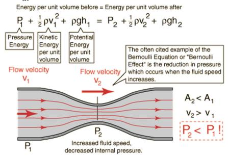
A special form of the Euler's equation derived along a fluid flow streamline is often called
