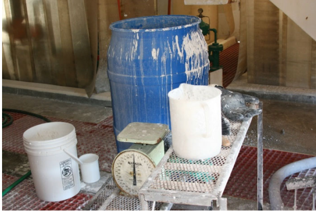
This photograph shows the containers of Lime slurry that was removed from the equipment after being placed out of service. The Lime had already hardened.
