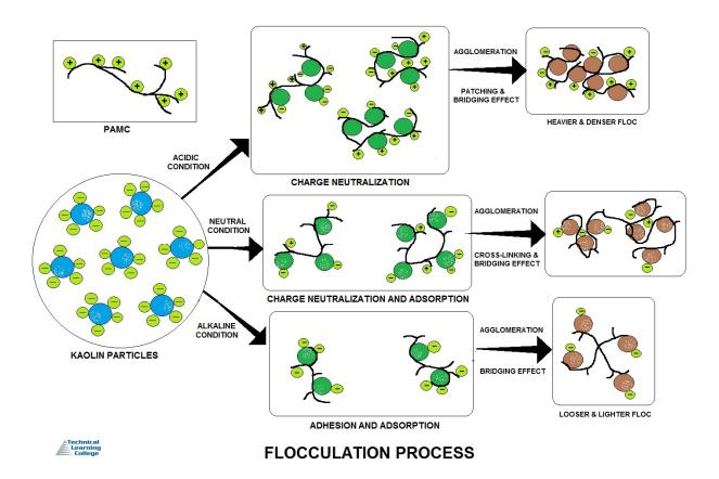
Activated sludge flocs are a flocculated mass of microorganisms, extracellular polymeric substances (EPS) and adsorbed organic and inorganic material. The structure of the floc is very heterogeneous and flocs with very different properties and morphologies may occur, depending on the conditions in the activated sludge treatment plant and wastewater composition.
