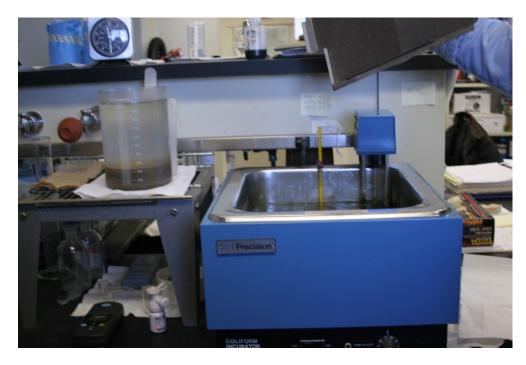
An incubator bath for the coliform test. The operator will place the sample in this device for 24 to 48 hours depending on the desired tests. There are several different methods to calculate coliform bacteria. This is an older true-and-tested method.
