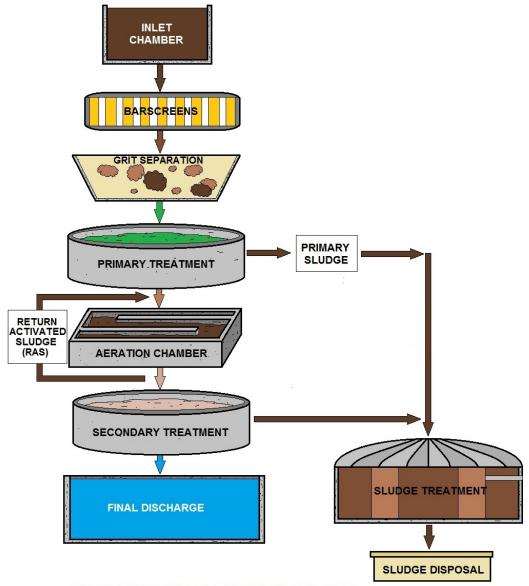
WASTEWATER TREATMENT PLANT (SLUDGE REMOVAL BASICS)
