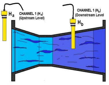
SUBMERGED FLOW SELECTION USES BOTH INPUT CHANNELS PER APPLICATION. THE SUBMERGED FLOW USES THE MEAUSUREMENT OF BOTH AN UPSTREAM LEVEL (Ha) AND A DOWNSTREAM LEVEL (Hb) TO DETERMINE THE ACTUAL FLOW RATE IN THE FLUME. THIS IS REFERRED AS SUBMERGENCE (Ha/Hb)
