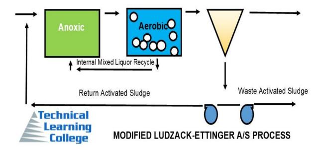
The Modified Ludzack-Ettinger (MLE) process developed for the combination removal of BOD, ammonia, and nitrate/nitrite. The process employs a combination of an anoxic and aerobic zone.
