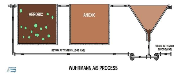
The Wuhrman process was first suggested in 1964. This process depended upon post denitrification using a secondary anoxic reactor following the aerobic zone.
