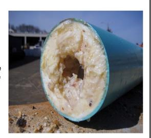
Onsite septic systems also can be harmed by too much fat, oil and grease, which can clog onsite system drainfield pipes and soils, adding to the risk of system failure. Excessive grease also adds to the septic tank's scum layer, causing more frequent tank pumping to be required. Both conditions can result in significant costs to homeowners.
