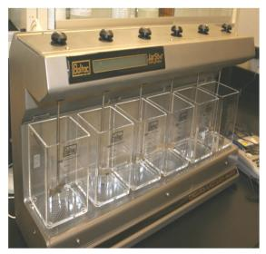
Jar Testing Apparatus
