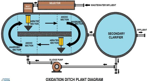
In the typical oxidation ditch, mixed liquor is pumped around an oval or circular pathway by brushes raptors or other mechanical aeration devices as well as pumping equipment located at one or more points along the flow path.
