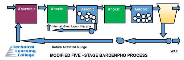
The Bardenpho process was named after its inventor, Dr. James Barnard. His process may be configures with four or five stages. The major difference process is that the Bardenpho process includes an anaerobic zone. Most of the treatment facilities that utilize this process have required supplemental chemical addition (metal salts and/or carbon) to meet the effluent phosphorus limits of less than 1.0 mg/L as P.
