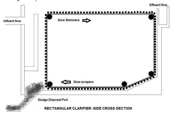
Let's look at the components of a rectangular clarifier. Most are designed with scrapers on the bottom to move the settled activated sludge to one or more hoppers at the influent end of the tank. It could have a screw conveyor or a traveling bridge used to collect and move the sludge along in the end hopper.
