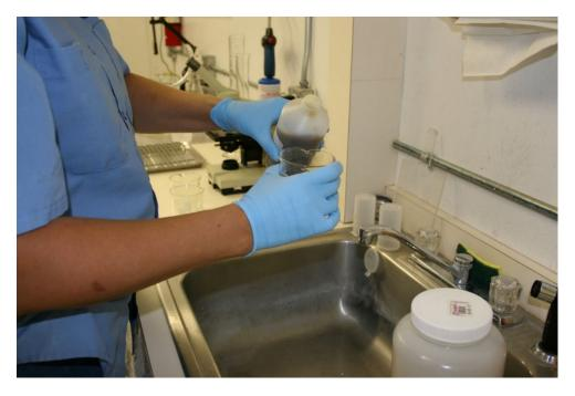
This operator is splitting the sample for bacteriological analysis. Always wear gloves for your and others' safety. We have all seen the operator who holds a sandwich in one hand while working in the lab, or the operator who does not wear gloves at all.
