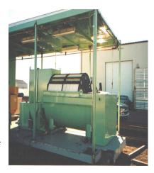
Rotating biological contactors can be supplied as part of an integral package plant to treat sewage from various communities. Integral units are provided in sizes of up to a 500-population equivalent. A smaller version is also available for small private installations.
