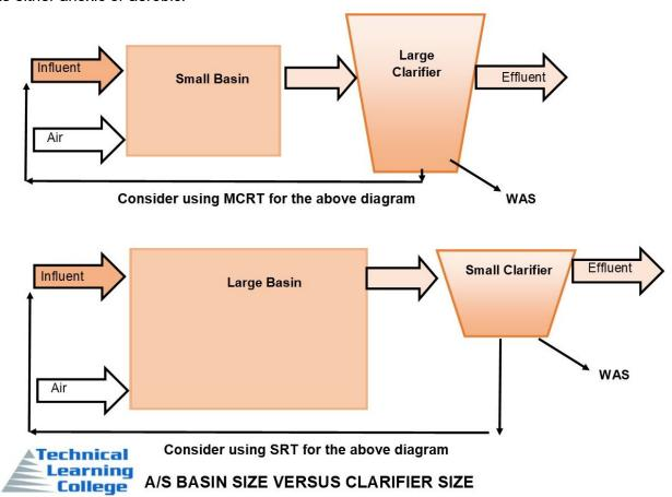
For a facility that has small activated sludge basin(s) and large clarifier(s), MCRT may be more appropriate because even when the clarifier sludge blanket is below 0.6 m (2 ft) of depth, a significant portion of the MLSS may be in the clarifier.
