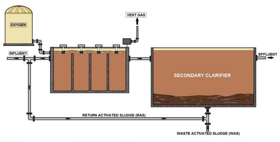
HIGH PURITY OXYGEN PLANT DIAGRAM
