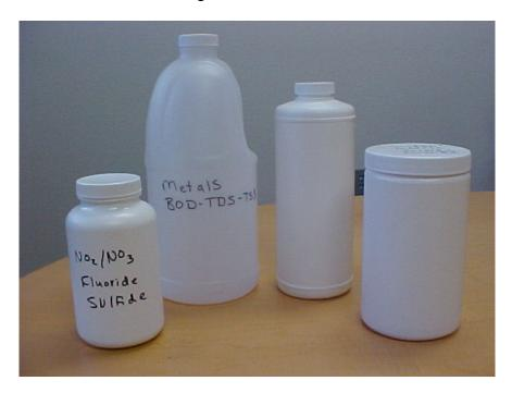
NO<sub>2</sub>/NO<sub>3</sub>, Fluoride, Sulfide, Metals, BOD-TDS-TSS Wide-mouth Sludge/Metals bottle
