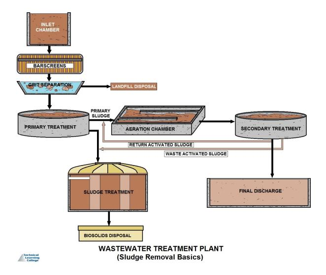
There are various options for treating sludge including stabilization, thickening, dewatering, drying, and incineration. The costs for treating sludge and removing sludge from wastewater are roughly the same. Typically a polymer chemical is used for the volume reduction process known as dewatering. Polymers are slippery chemicals, which means that there is always a risk of slipping or falling due to spills and leaks. Polymers can also be environmental stress crack agents.
