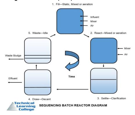
The SBR process is a sequential suspended growth (activated sludge) process in which all major steps occur in the same tank in sequential order (USEPA, 2008d). The SBR system is typically found in packaged configurations for onsite and small community or cluster applications. The major components of the package include the batch tanks, aerator, mixer, decanter device, process control system (including timers), pumps, piping, and appurtenances.
