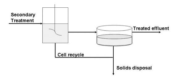
Diagram of a simple activated sludge system.
