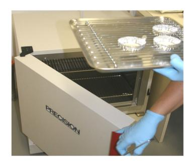
These filters (cookies) contain samples from the primary influent that are lighter than activated sludge samples
