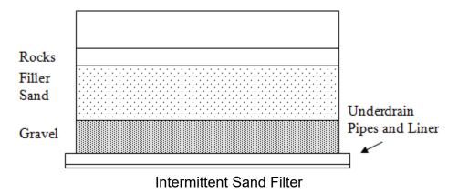
ISFs are aerobic, fixed-film bioreactors. Bioslimes from the growth of microorganisms develop as films on the sand particle surfaces. The microorganisms in the slimes capture soluble and colloidal waste materials in the wastewater as it percolates through the sand surfaces. The captured materials are metabolized into new cell mass or degraded under aerobic conditions to carbon dioxide and water.
