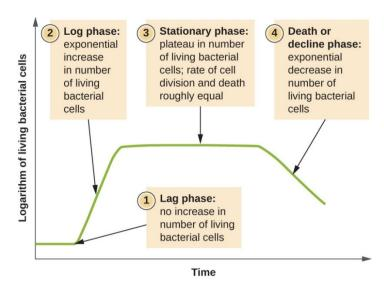
The graph above illustrates the growth phases in a biological system and how the growth rate of microorganisms' changes with increased CRT.
