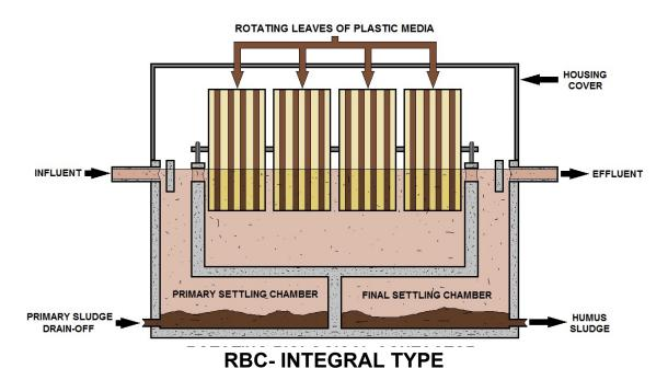
RBC's with integral units treat unsettled sewage and has the capability of providing primary and secondary settling in the unit.
