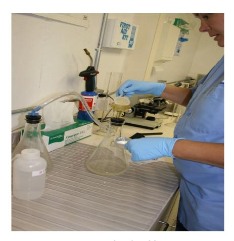
Lab tech removing filter for TSS analysis.
