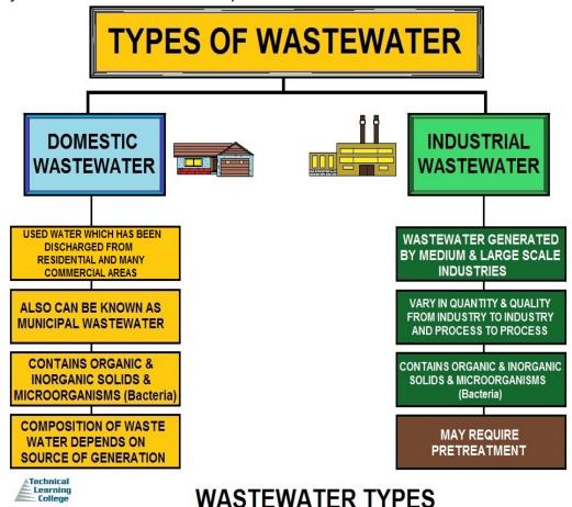
The diagram above shows the difference between domestic wastewater and industrial wastewater. Not all communities have industrial waste and if they do, the plant generally treats a high volume of flow.
