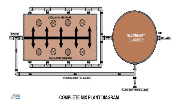
In a complete mix activated sludge process, the mixed liquor is similar throughout the aeration tank. The operating characteristics in terms of solids, oxygen uptake rate (OUR), MLSS, and soluble  $BOD_5$  concentration are identical throughout the tank.
