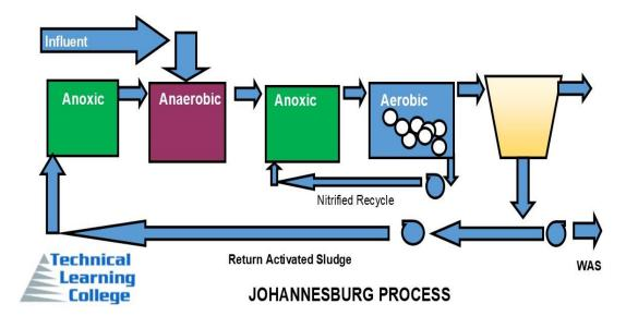
The JHB process is similar to the 3 Stage Pho-redox process, but has a pre-anoxic tank ahead of the anaerobic zone to protect the zone from nitrates when low effluent nitrates are not required. The low COD of the wastewater limited the de-nitrification capacity in the original plant (Northern Works), resulting in nitrates in the RAS.
