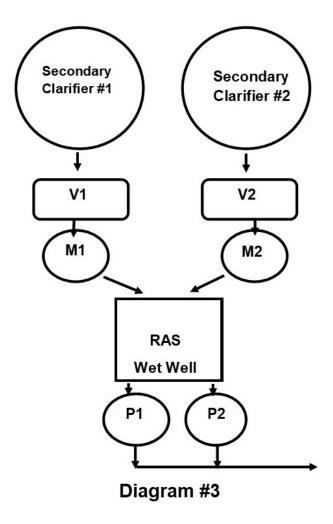
Diagram # 3 represents the best approach. RAS from each clarifier flows through a control valve and flow meter to a wet well, where a set of pumps draws from the wet well. This arrangement allows the operator to make adjustments to the RAS flow from each clarifier as needed. If the common RAS flow goes to separate aeration tanks, then separate control valves and meters for each tank should also be part of the system.
