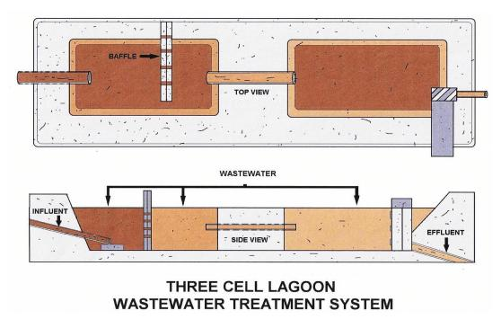
Lagoon systems consist of aerated cells, followed by a non-aerated polishing cell and a final chlorine contact chamber. Often flowed by a non-aerated cell for sludge settling.
