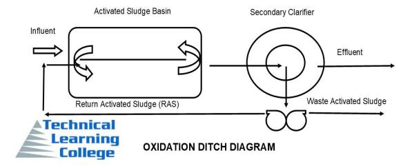
There are several oxidation ditch designs that can remove phosphorus. They normally consist of an anaerobic zone ahead of the oxidation ditch, whereas simultaneous nitrification and denitrification takes place within the ditches.
