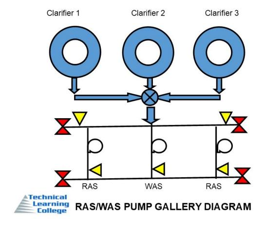
The advantage of pulling MLSS from the bottom of the clarifier or RAS line instead of the activated sludge basin is that the RAS will have a higher concentration in milligrams per liter. This reduces the total volume that must be removed and processed.
