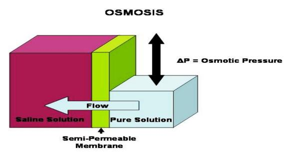
The semi-permeable membrane is so designated because it permits certain elements to pass through, while blocking others. The elements that pass through include water, usually smaller molecules of dissolved solids, and most gases. The dissolved solids are usually further restricted based on their respective electrical charge.
