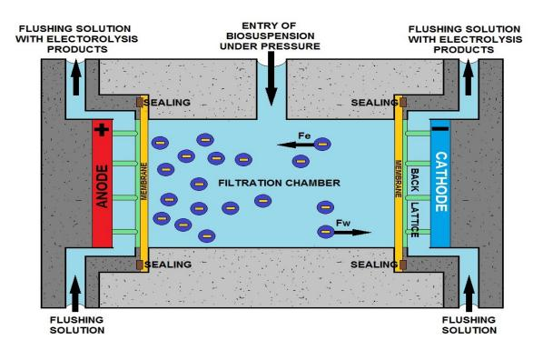
**ELECTROFILTRATION CHAMBER DIAGRAM**
