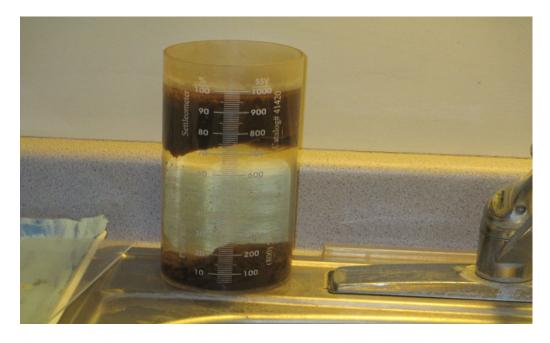
During the settleometer test, operators not only check how the solids settle out they can also determine the rate of denitrification in the clarifier. This rising sludge is the result of denitrification.
