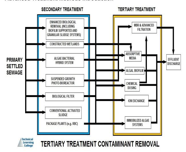
In advanced wastewater treatment, methods are dependent upon the characteristics of effluent to be obtained after secondary treatment to satisfy further use or disposal of treated wastewater. The diagram above list different methods depending on the removal of BOD, TSS and minor portions of nitrogen, phosphorus, and heavy metals achieved during secondary treatment.
