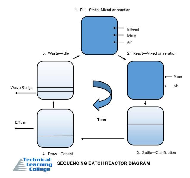
Sequencing batch reactors (SBR) or sequential batch reactors are industrial processing tanks for the treatment of wastewater. SBR reactors treat wastewater such as sewage or output from anaerobic digesters or mechanical biological treatment facilities in batches. Air or oxygen is bubbled through the wastewater to reduce biochemical oxygen demand (BOD) and chemical oxygen demand (COD) to make suitable for discharge. While there are several configurations of SBRs the basic process is similar.
