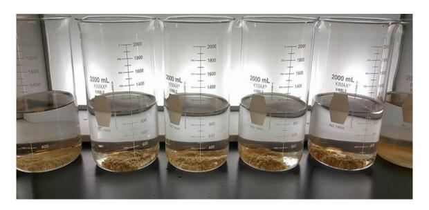
Well-formed coagulated floc results after settling.
