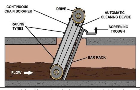
The bar rack consist of parallel bars, rods, or wires (coarse screen) or perforated pipe (fine screen).
