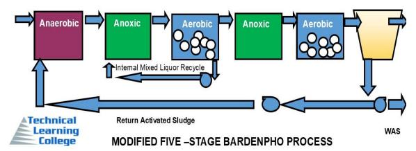
The Bardenpho process removes nitrogen to low concentrations. The addition of an anaerobic zone at the head of the process enables phosphorus removal as well. The process consists of 5 stages: an anaerobic stage followed by alternating anoxic and aerobic stages. A nitrate-rich liquor is recycled from the first aerobic stage, designed for complete nitrification, to the first anoxic stage.
