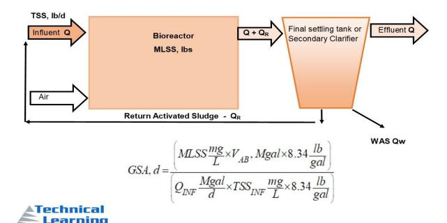
GOULD A/S SLUDGE FLOW DIAGRAM AND FORMULA
