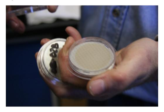
This is a filter used for the coliform test.
