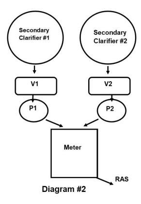
If we divide the meter reading in half, will we get the flow rate for each clarifier? In diagram #2, each clarifier has its own RAS flow control valve and pump. The two pumps discharge into a common pipe where the flow is metered. This is a better situation, allowing the operator to vary the amount of RAS from each clarifier, but since the meter only measures the total flow from the two clarifiers, it will be very difficult to balance the RAS flow.
