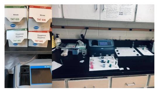
HACH DR 3900 is a widely used spectrophotometer to determine multiple analyses or parameters. The vial with the bluish coloration (center) is phosphorus.
