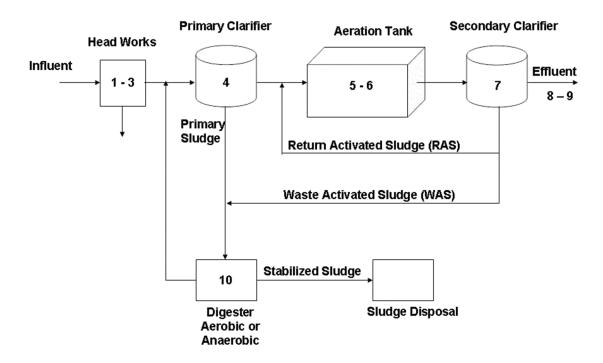
Air is necessary at process number 5-6.
