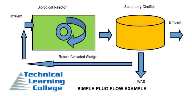
As a result, the concentration of BOD and the oxygen usage will decrease along the basin length. The BOD will decrease, MLSS and MLVSS will increase along the basin length as biomass is produced. This type of flow is approximated by long, narrow basins with length-to-width ratios greater than 10. That is, the basins are at least 10 times longer than they are wide.
