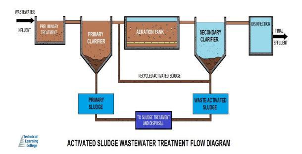
The nitrification process requires a slow-growing nitrifying bacteria with sludge that has been aged for a long time and high dissolved oxygen concentration. In addition, they were susceptible to inhibition by a wide range of compounds at concentrations so low as not to affect the heterotrophic bacteria. For these reasons, it would seem sensible to separate the processes of carbonaceous removal and nitrogen removal into separate reactors (Horan, 1989).
