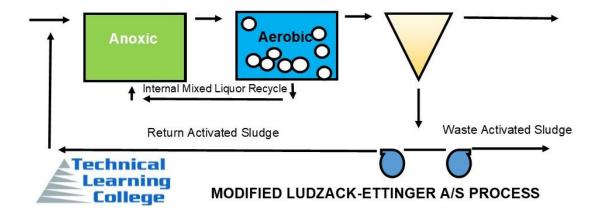
The most common nitrogen removal process used at WWTPs is the Modified Ludzck Ettinger (MLE) process, which is considered a pre-denitrification, single sludge system. The process includes an initial anoxic zone, followed by an aerobic zone.
