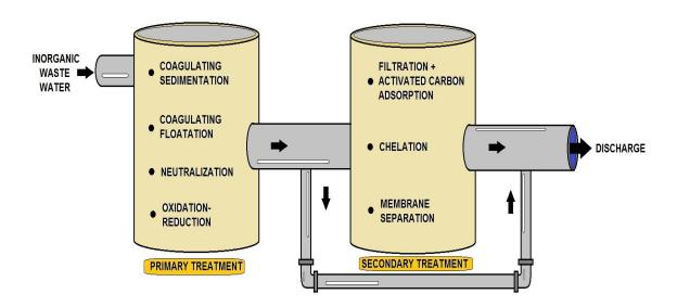
PROCESS OF REMOVING INORGANIC WASTE (Flow Diagram)
