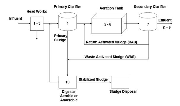
Microlife's health is essential for the proper operation of box 5, 6, 7 and 10. Box 4 is for settling of the solids.
