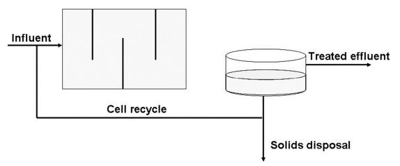
Diagram of a conventional activated sludge process.
