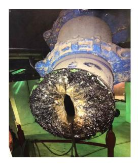
Struvite deposits inside a digester pipe.
