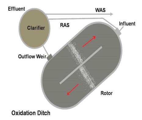
Many times in plants that have advanced treatment methods, we as operators will send RAS to the oxidation ditch or lagoon to eat the raw food in the system.
