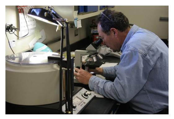
Optical microscopes are used to see indicator bugs and other microorganisms. This examination is used so that the operator knows how well the process is working.
