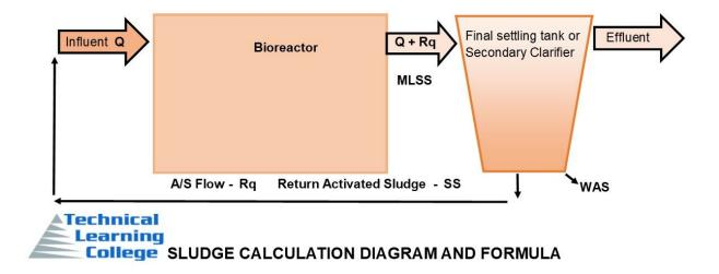
This approach is centered on the thought that in a secondary clarifier the pounds of solids drawn from the clarifier (RAS) must be equal to the pounds of material entering the clarifier (MLSS).
