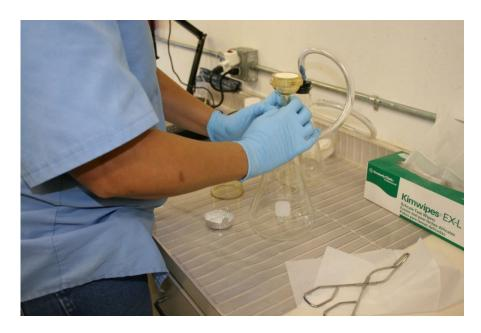
**Total dissolved solids** - The weight per unit volume of all volatile and non-volatile solids dissolved in a water or wastewater after a sample has been filtered to remove colloidal and suspended solids. The lab tech is filtering a wastewater sample.
