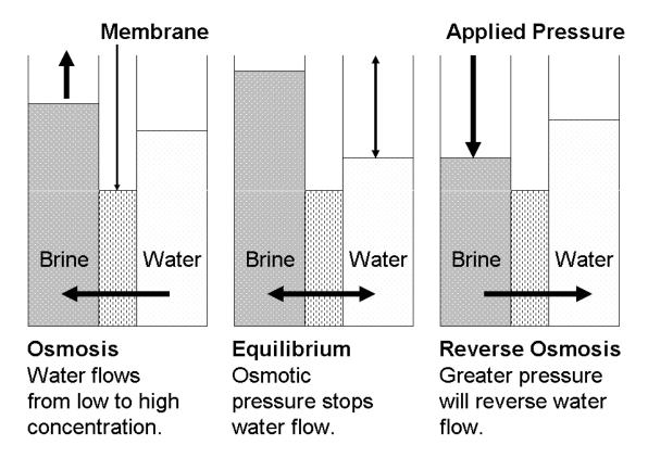
The membrane must be physically strong to stand up to high osmotic pressure - in the case of sea water, 2500 kg/m. Most membranes are made of cellulose acetate or polyamide composites cast into a thin film, either as a sheet or fine hollow fibers. The membrane is constructed into a cartridge called a reverse osmosis module.
