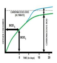
ONE REASON TO USE INCUBATION PERIOD OF 5 DAYS FOR BOD DETERMINATION, IS TO ELIMINATE OXYGEN DEMAND FOR NITRIFICATION, THEREFORE TO FIND OUT ONLY THE CARBONACEOUS OXYGEN DEMAND (BOD5 / BODu = 0.68)
