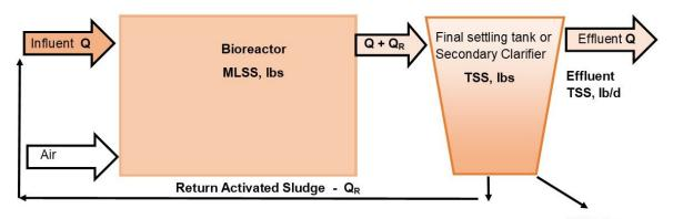
$$MCRT, d = \frac{\left(V_{AB}, Mgal \times MLSS\frac{mg}{L}\right) + \left(V_{SC}, Mgal \times TSS_{SC}\frac{mg}{L}\right)}{\left(Q_{WAS}\frac{Mgal}{d} \times TSS_{WAS}\frac{mg}{L}\right) + \left(Q_{EFF}\frac{Mgal}{d} \times TSS_{EFF}\frac{mg}{L}\right)}$$
