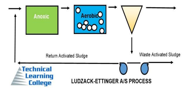
In the early 1970's, James Barnard suggested the addition of a mixed liquor recycle to return nitrate back to the anoxic zone, and named the process Modified Ludzack Ettinger. The MLE is regarded as the first successful nitrogen removal activated sludge process.
