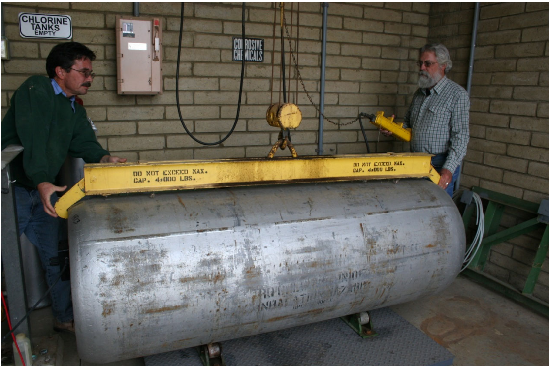
Top photograph, a view of the top of a 150 gas cylinder. Bottom, always work in pairs when working around Chlorine. Here the hoist is being used to move the container.
