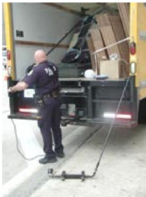
Obstructed Cargo Area Search w/Pole. Quick Connect Trolley For Under Vehicle Search (in foreground)
