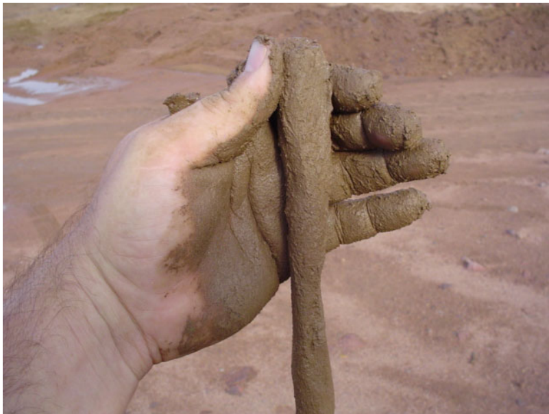
Ribbon Soil Test
