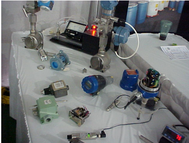
Examples of various sewer flow measuring devices
