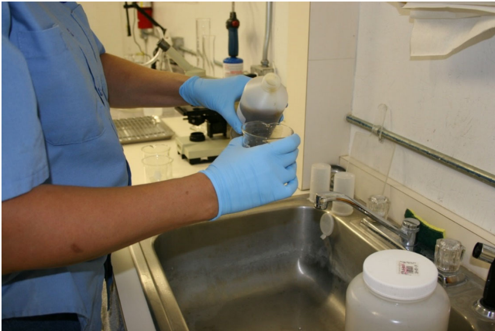
This operator is splitting the sample for bacteriological analysis. Always wear gloves for your and others' safety. We have all seen the operator holds a sandwich in one hand while working in the lab, or the operator does not wear gloves at all.
