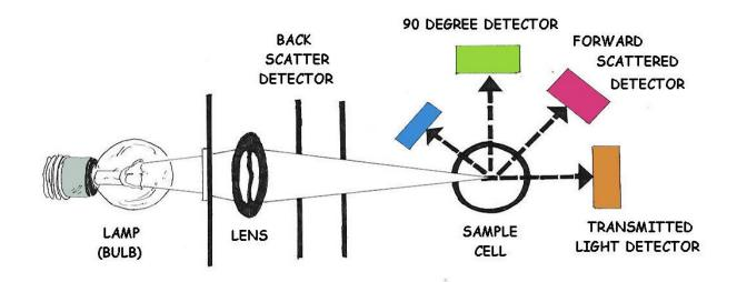
HOW AN TURBIDIMETER WORKS
