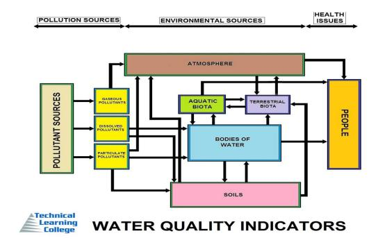
Because raw water (surface water) is never pure of pollution, we need to properly treat it. Most of the earth's water sources obtain their water supplies through precipitation (rain). During precipitation, water passes over (runoff) and through the ground (infiltration), acquiring a wide variety of dissolved or suspended impurities that intensely alters its usefulness. Water has unique physical, chemical and biological properties.
