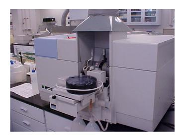
Gas Chromatograph Used for micro-contaminant water analysis.
