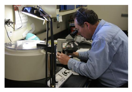
Phase microscopes are used to see indicator bugs and other MO's microorganisms. This examination is used so that the operator knows how well the process is working.
