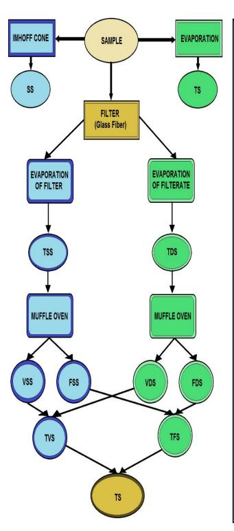
**FSS: Fixed Suspended Solids TDS: Total Dissolved Solids VDS: Volatile Dissolved Solids** FDS: Fixed Dissolved Solids TVS: Total Volatile Solids **TFS: Total Fixed Solids EQUIPMENT USED TO MEASURE AND DETERMINE TYPES OF SOLIDS**
