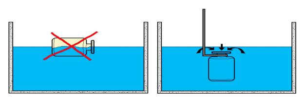
PROPER MATHOD OF TAKING IMMERSE TYPE WATER SAMPLES.
