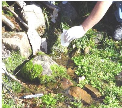
Sampling downstream from a wastewater plant's discharge point.
