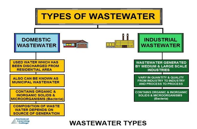
The diagram above shows the difference between domestic wastewater and industrial wastewater. Not all communities have industrial waste and if they do, the plant generally treats a high volume of flow.
