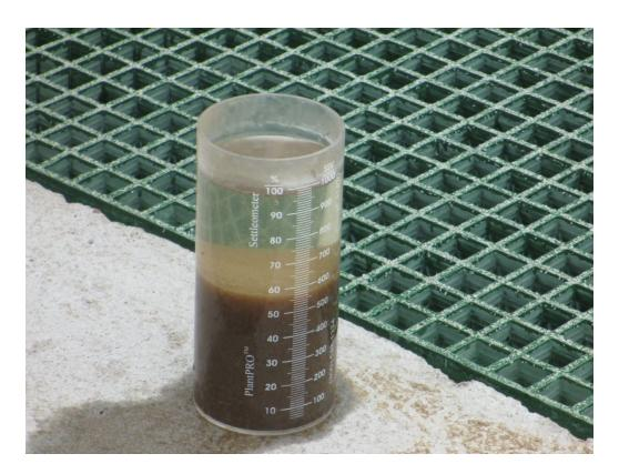
The settleometer is a great tool for operators. It indicates how the solids will settle in the clarifier and the density of the sludge.
