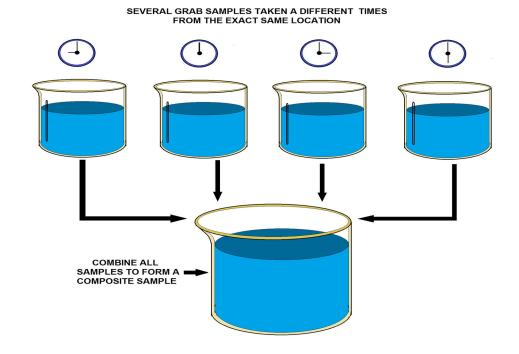
MAKING A COMPOSITE SAMPLE FROM GRAB SAMPLES DIAGRAM
