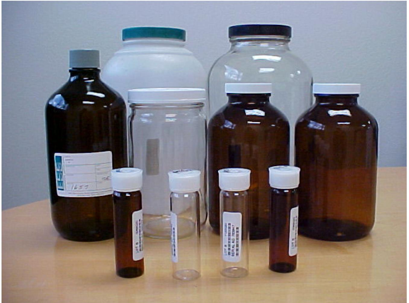
Common wastewater sampling bottles. SOC/VOC bottles are the smaller, thin bottles with the septum tops. Be careful not to get any air bubbles in the SOC/VOC bottles
