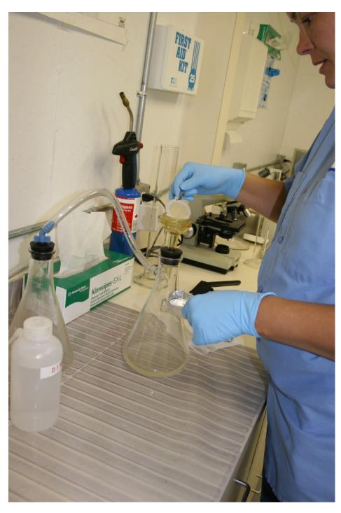
Lab tech removing filter for TSS analysis.
