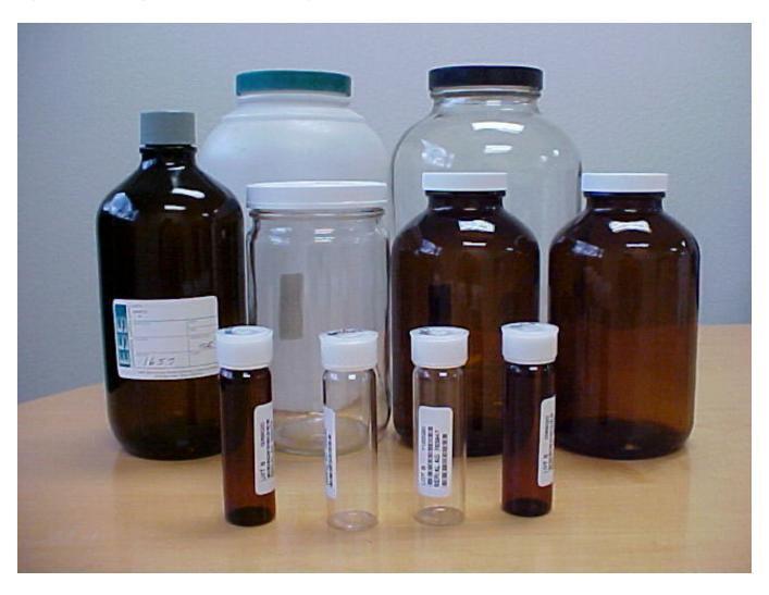
Common wastewater sampling bottles. SOC/VOC bottles are the smaller, thin bottles with the septum tops. Be careful not to get any air bubbles in the SOC/VOC bottles
