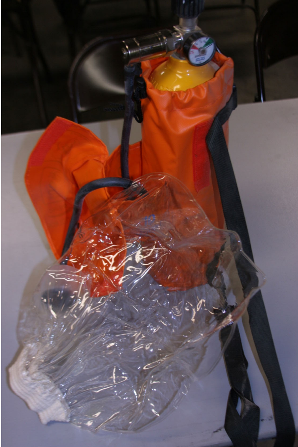
A ten-minute escape air pack. Enough air for you to escape out of a hazardous atmosphere. There are smaller versions of this device.
