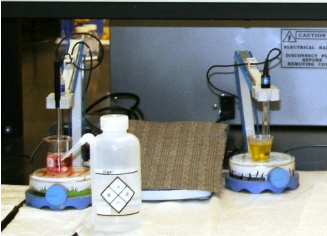
Common pH measurement equipment and probe rinse agent in plastic bottle.
