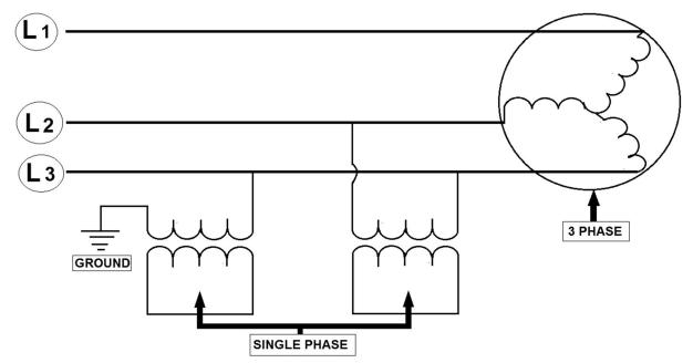
Three-phase electricity powers large industrial loads more efficiently than single phase electricity. When- single-phase electricity is needed, it is available between any two phases, or, in some systems, between one of the phases and ground.
