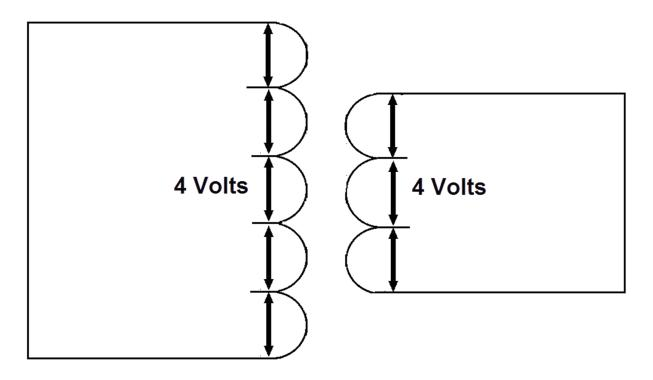
Most transformers are designed either to step voltage up or to step it down, although some are used only to isolate one voltage from another.
