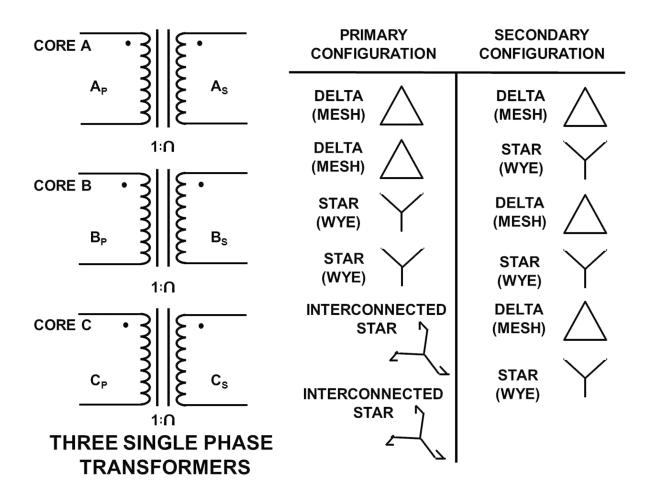
The primary and secondary windings of a transformer can be connected in different configuration as shown to meet practically any requirement. In the case of *three phase transformer* windings, three forms of connection are possible: "star" (wye), "delta" (mesh) and "interconnected-star" (zig-zag).
