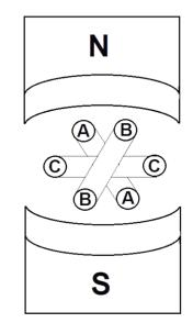
As the coils turn through the magnetic field, power is sent out on three lines. Three current and voltage sine waves are generated, 120 degrees out of phase with each other. Each sine wave represents the current or voltage on one of the phases.
