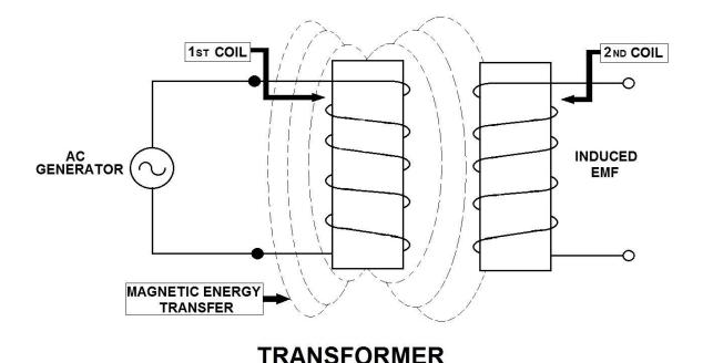
A transformer most commonly consists of two windings of wire wound around a common core to effect tight electromagnetic coupling between the windings. The core material is often a laminated iron core. The coil that receives the electrical input energy is referred to as the primary winding, while the output coil is called the secondary winding.
