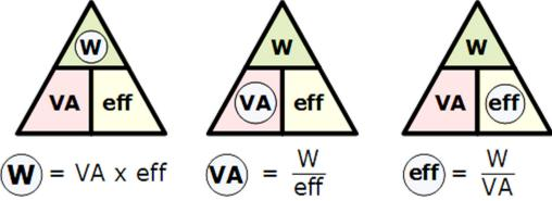
Then, to find Watts (output) = VA x eff., or to find VA (input) = W/eff., or to find Efficiency, eff. = W/VA, etc.
