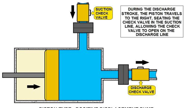
PISTON TYPE – POSITIVE DISPLACEMENT PUMP
