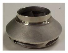
**Closed Pump Impeller**
