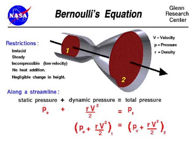
Here is where Bernoulli's equation figures in. As the water slows down and its kinetic energy decreases, that water's pressure potential energy increases (*to conserve energy*). Thus, the slowing is accompanied by a pressure rise.
