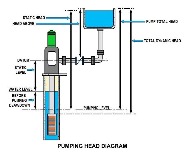
NPSH is initialism for Net Positive Suction Head. In any cross-section of a generic hydraulic circuit, the NPSH parameter shows the difference between the actual pressure of a liquid in a pipeline and the liquid's vapor pressure at a given temperature.
