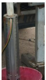
The PVC pipe id threaded into the pump assembly. The PVC is special pre-threaded pipe.
