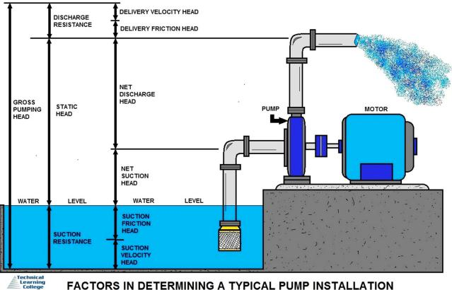
FACTORS IN DETERMINING A TYPICAL PUMP INSTALLATION
