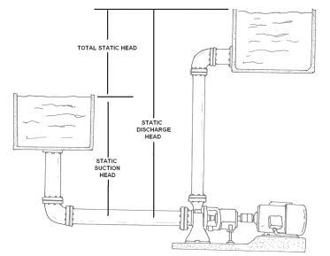
caused by water moving through the hose or pipes. Dynamic indicates that losses due to friction are factored into the performance. The following terms are usually used when referring to lift or head.
