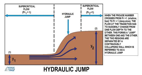
A hydraulic jump is a phenomenon in the science of hydraulics which is frequently observed in open channel flow such as rivers and spillways. When liquid at high velocity discharges into a zone of lower velocity, a rather abrupt rise occurs in the liquid surface. Hydraulic jump is the jump or standing wave formed when the depth of flow of water changes from supercritical to subcritical state.
