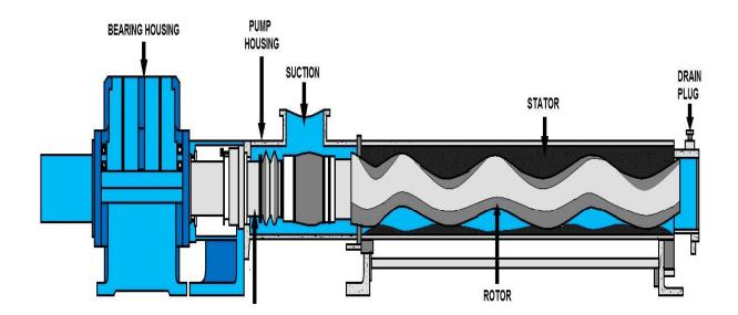
POSITIVE DISPLACEMENT PUMP PROGRESSIVE CAVITY TYPE
