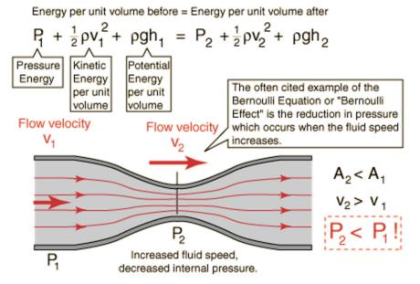
A special form of the Euler's equation derived along a fluid flow streamline is often called the **Bernoulli Equation.**
