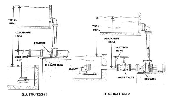
Here are the important points to consider about suction piping when the liquid being pumped is below the level of the pump:
