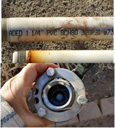
Looking at the discharge side of the pump where the pipe is screwed in and you can see the foot valve on the inside.
