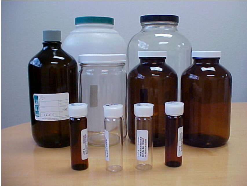
625/608, 1657, TTO/Organics, TPH/Oil/Grease, Thin vials-TOCs, VOCs, 601/602 and 502.2 Be careful not to get air in the VOC/SVOC bottles.
