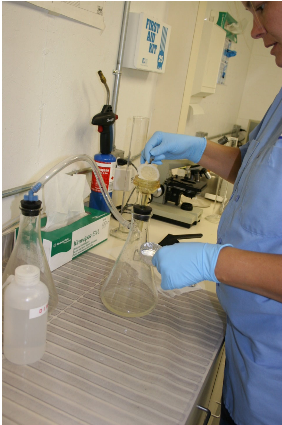
Lab tech removing filter for TSS analysis.
