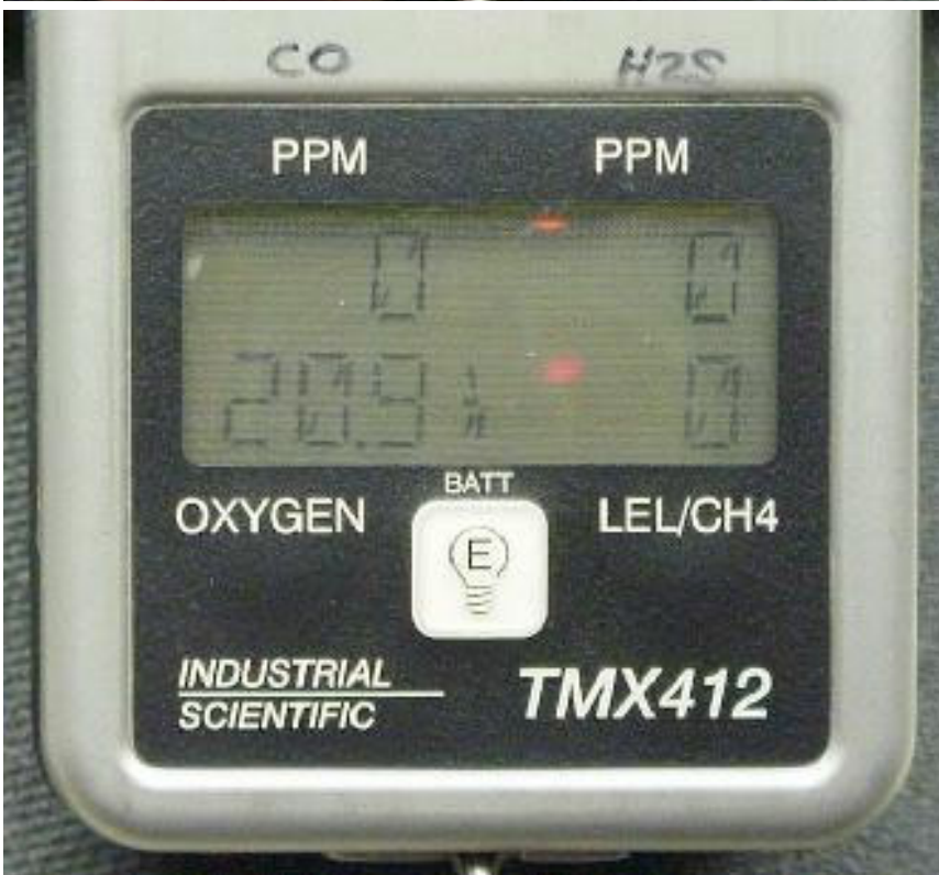
Example of a clean air display. Carbon monoxide ( CO ) and hydrogen sulfide ( H 2 S ) are in ppm; oxygen ( O 2 ) and lower explosive limit ( LEL ) readings are percentage values. The battery-life indicator is just right of the oxygen display (i.e., 20.9); each line represents about one hour of service remaining.
