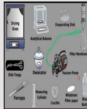
EQUIPMENT USED TO MEASURE AND DETERMINE TYPES OF SOLIDS
