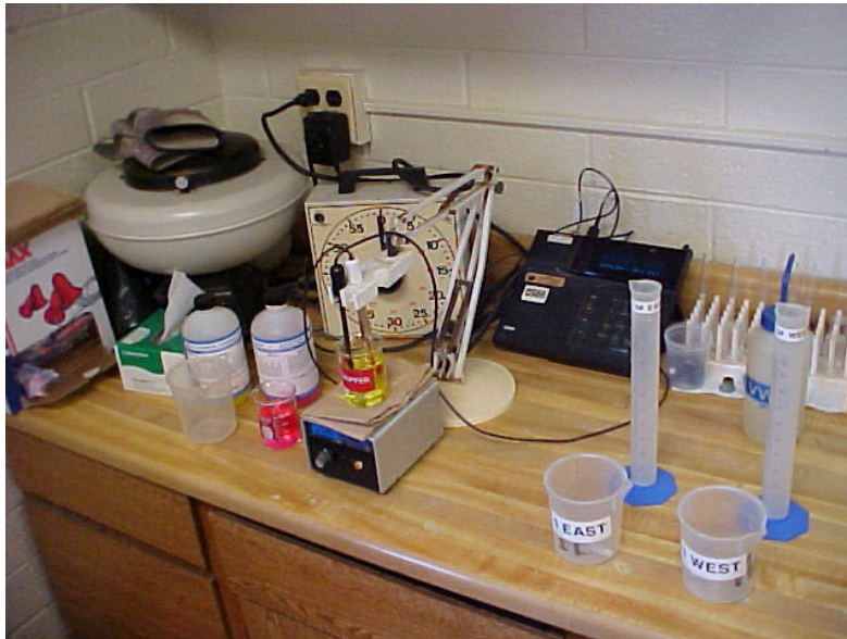
A small wastewater treatment plant operator's lab with a centrifuge, timer, pH meter, standard buffer solutions and settling beakers.
