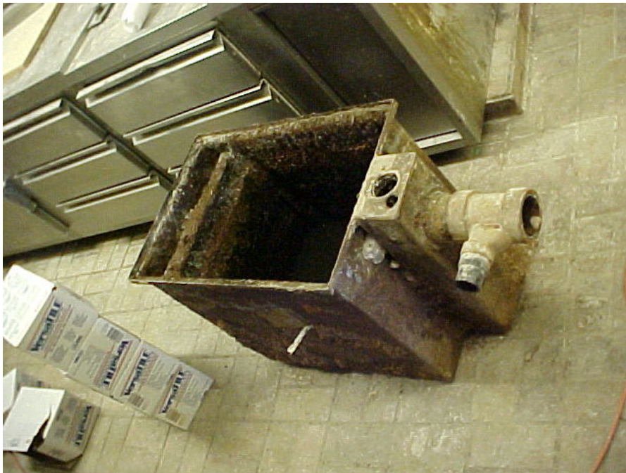
Common and worn out kitchen Grease Trap. The grease contains lots of acid and this acid will eat metal as with this grease trap.
