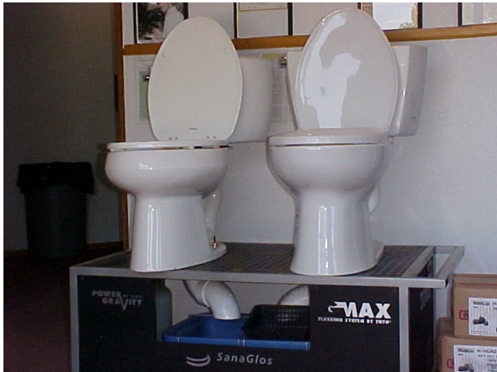
Testing 1.6 gallon toilets against each other. Toilet retrofit programs have save thousands of gallons of water.
