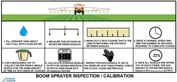
Use maximum gallonage (3 gallons spray or more by air or 6 gallons/acre with ground equipment) per acre and low pressure (max 25 PSI for aircraft and 40 PSI for ground sprayers).
