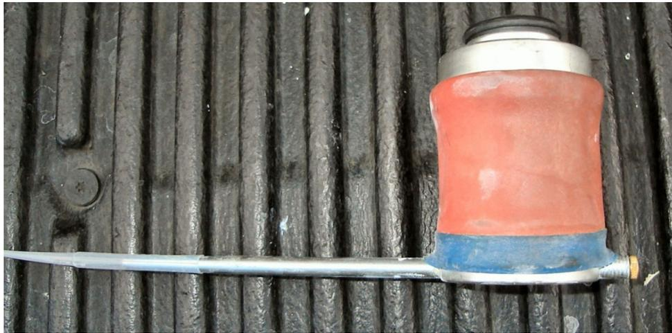
The above photograph is a **Crusader Duster** or dust applicator and is great for voids in walls or cracks and crevices. Just pour your product in the top and squeeze the product into the cracks or inside switch plates. You have to get in the pest's home to kill them! Notice the plastic tip so that you do not get an electric shock. This moneymaking tool is great to kill cockroaches, bees or termites. Cockroaches are one of the easiest to kill if you can get product on them.
