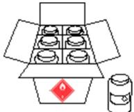
Figure 4.13 Combination Packaging (Outer box with inner bottles)
