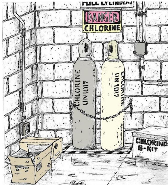
**Safety Information:** There is a fusible plug on every chlorine gas cylinder. This metal plug will melt at 158° to 165° F. This is to prevent a build-up of excessive pressure and the possibility of cylinder rupture due to fire or high temperatures.
