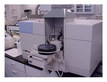
Gas Chromatograph Used for micro-contaminant water analysis.
