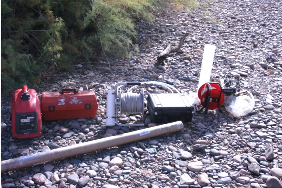
Top Photo: Technicians use several different devices to sample wells depending on the depth of the water table. Some use hand bailers or small gas powered submersible pumps.
