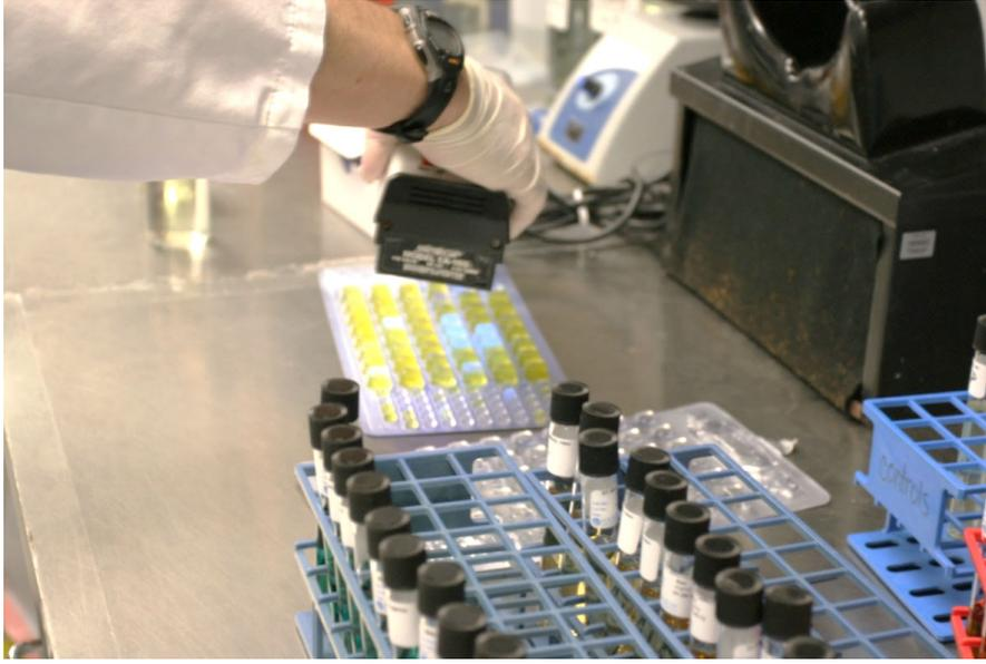
Top Photo: This technician is using Colilert which is a commercially available enzyme-substrate liquid-broth medium (IDEXX Laboratories, Inc.) that allows the simultaneous detection of total coliforms and *Escherichia coli* (*E. coli*). It is available in the most-probable number (MPN) or the presence/absence (PA) format. The MPN method is facilitated by use of a specially designed disposable incubation tray called the Quanti-Tray®.
