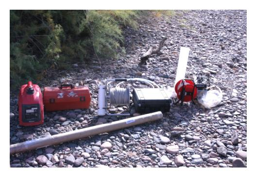
Top Photo: Technicians use several different devices to sample wells depending on the depth of the water table. Some use hand bailers or small gas powered submersible pumps.
