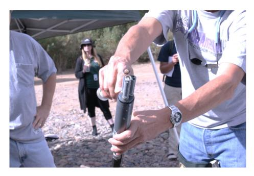
Top Photo: This multi probe device measures dissolved oxygen (DO), pH, conductivity and total dissolved solids (TDS), the device requires calibration for each parameter.
