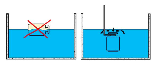
PROPER MATHOD OF TAKING IMMERSE TYPE WATER SAMPLES.
