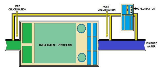
CHLORINE FLOW IN A TREATMENT PLANT
