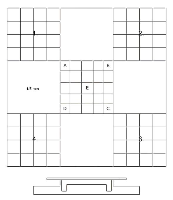
Hemacytometer Platform Ruling. Squares 1, 2, 3, and 4 are used to count stock suspensions of *Cryptosporidium* oocysts and *Giardia* cysts (after Miale, 1967)
