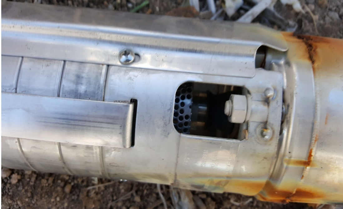
Pump and motor connection.
