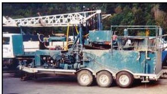
Small Self-Contained Mud System
