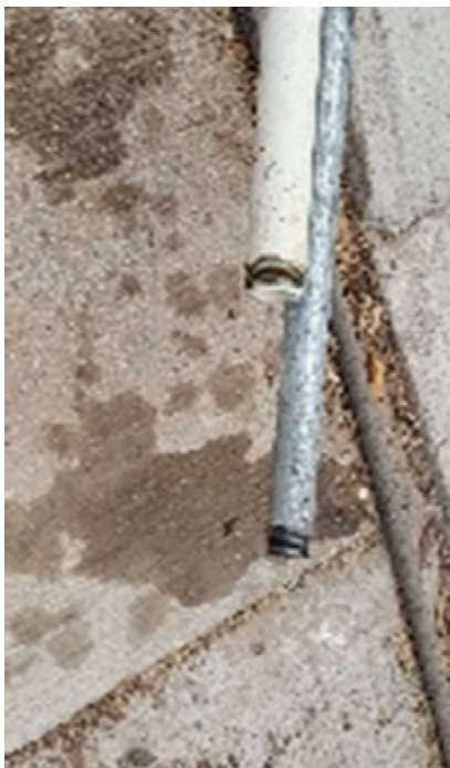
Attachment that screws into well pipe to be pulled. Metal disk supports couplings on wellhead while being pulled.
