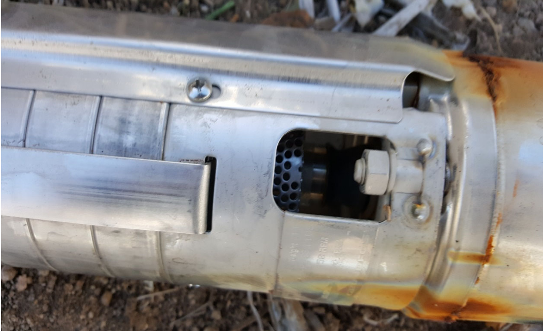
Pump and motor connection.
