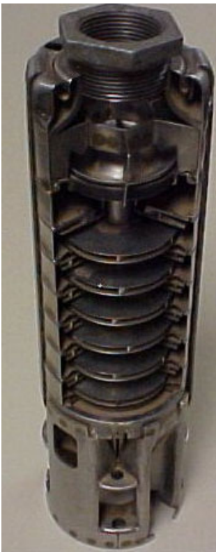
Cut away of a small submersible (turbine) pump without a motor.
