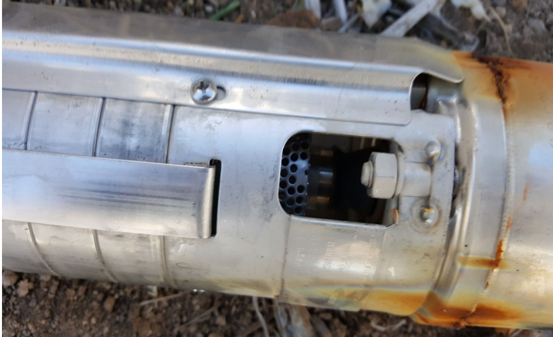
Pump and motor connection.
