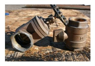
Flush the pipeline before installing the valve. Debris allowed to remain in the pipeline (such as weld spatters, welding rods, bricks, tools, etc.) can damage the valve. After installation, cycle the valve a minimum of three times and re-torque bolts as required. Ensure that the valve is in the open position and the inside of the body bore of the valve body/body end is coated with a suitable spatter guard.
