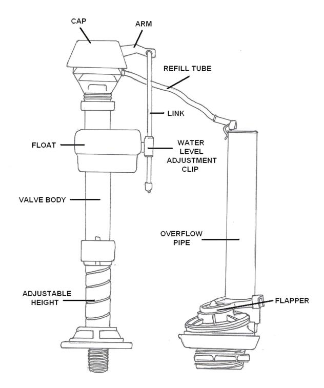
WATER CLOSET FLUSHING ASSEMBLY DIAGRAM
