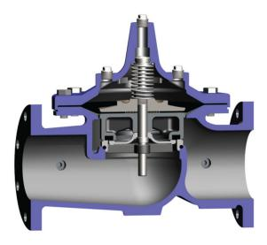
When no pressure is in the valve, the spring and the weight of the diaphragm assembly hold the valve closed.
