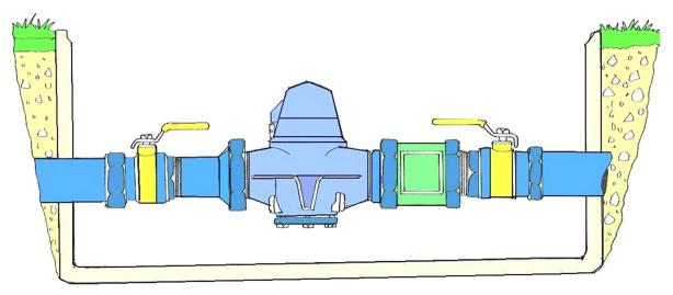
RESIDENTIAL DUAL CHECK VALVE INSTALLATION AT THE WATER METER
