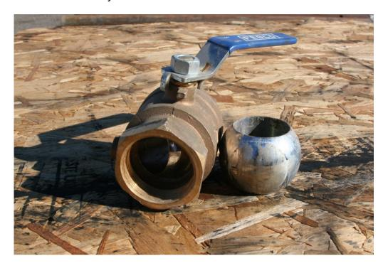
Removing the ball is very difficult. I think they use a robot to tighten the rear nut to keep you from removing it. I recommend that you always use pipe dope or Teflon tape when installing a Stop. I know a lot of you think that brass or bronze will make up the slack, but pipe dope, or Teflon dope or tape makes a nicer job and makes for an easier removal.
