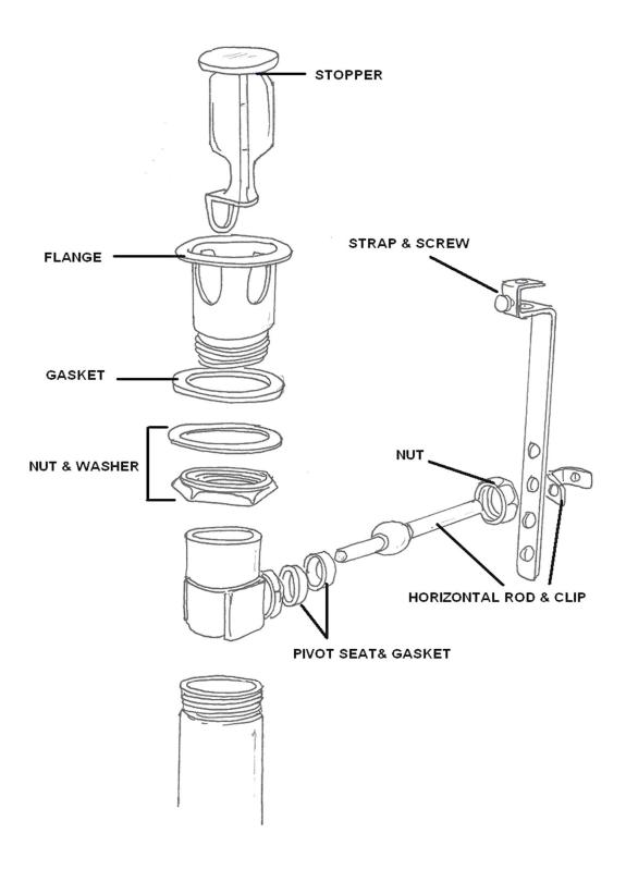
**BASIC DRAIN STOP PART DIAGRAM**
