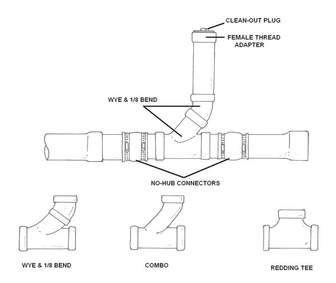
**SEWER WYE FITTING DIAGRAM**
