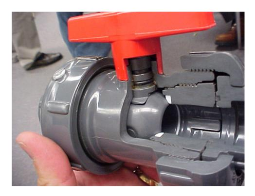
Upper, cut away of a Ball Valve. Below, cut away of a Gate Valve.
