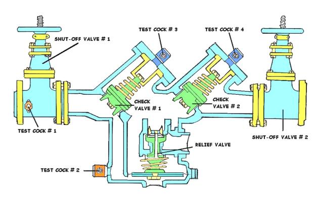
**REDUCED - PRESSURE PRINCIPLE BACKFLOW ASSEMBLY**
