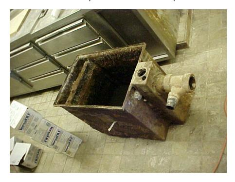
Common and worn out kitchen Grease Trap. The grease contains lots of acid and this acid will eat metal as with this grease trap.
