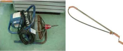
There are two basic snakes: 1) a closet auger with bent tip made to fit in a toilet's built in trap, 2) a drain auger which is a coiled rod or flattened metal strip.
