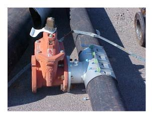
Gate Valves are used to isolate sections of water mains. Not to be used to throttle or regulate the flow.
