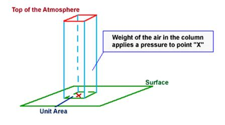
Pressure may be referred to using an absolute scale, pounds per square inch absolute (psia), or gauge scale, (psiag). Absolute pressure and gauge pressure are related. Absolute pressure is equal to gauge pressure plus the atmospheric pressure. At sea level, the atmospheric pressure is 14.7 psia.
