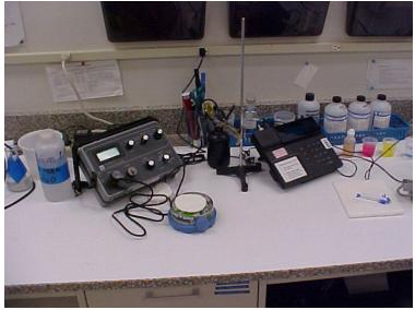
Commonly found conductivity, temperature and pH measuring equipment. As a sampler, you will use this equipment on a daily basis. Make sure to date the pH buffers and calibrate your equipment every morning.
