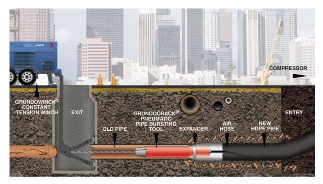
Cast iron and clay sewer lines often have more points of failure than high density polyethylene pipe or HDPE because they have more joints and joins. HDPE pipe is seamless, and so introduces fewer potential points of failure.
