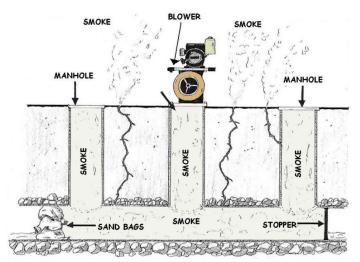
by a chemical reaction, creating a smoke which contains a high content of atmospheric moisture. It is very visible even at low concentrations, and extremely effective at finding leaks.
