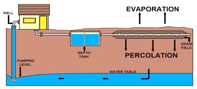
HOW SEPTIC TANK EFFLUENT PERCOLATES INTO THE WATER TABLE
