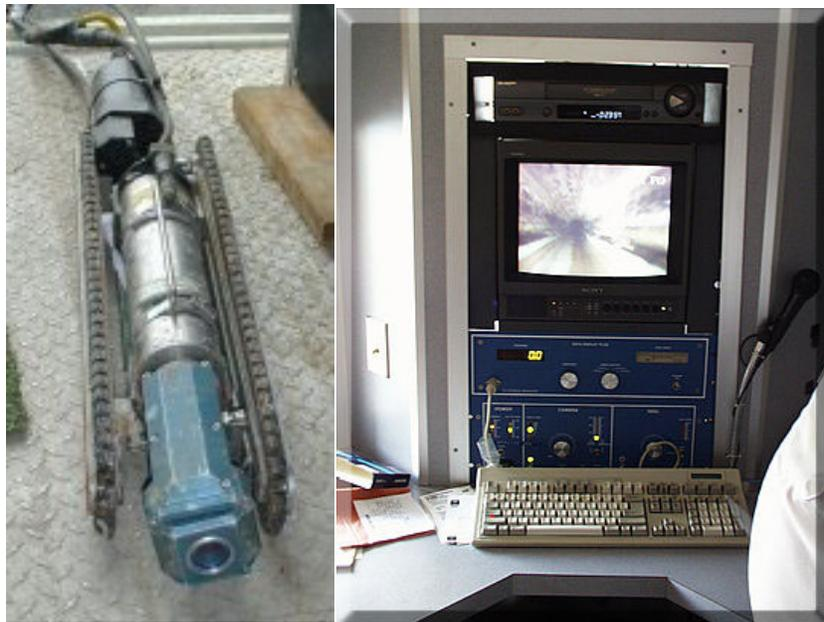
The Televising Van should be equipped with two cameras, one color camera for televising main sanitary lines and one color or black & white camera for televising house services (connection from the main sanitary line to a house).
