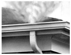
The smoke travels the path of least resistance and quickly shows up at sites that allow surface water inflow. Smoke will identify broken manholes, illegal connections (including roof drains, sump pumps, yard drains and more), uncapped lines, and will even shows cracked mains and laterals providing there is a passageway for the smoke to travel to the surface.
