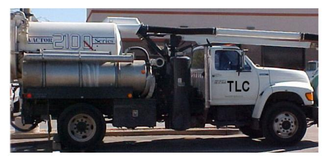
The sewer vacuum truck utilizes both a high pressure stream of water and a vacuum system to clean and remove built up debris from sewer lines. These versatile vehicles are also used to clean lift station wet wells, stormwater catch basins, and to perform excavations to locate broken water or sewer lines. It reduces repair times and costs by over 50%.
