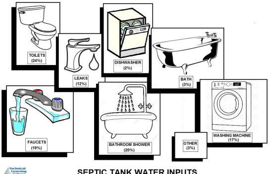
SEPTIC TANK WATER INPUTS
