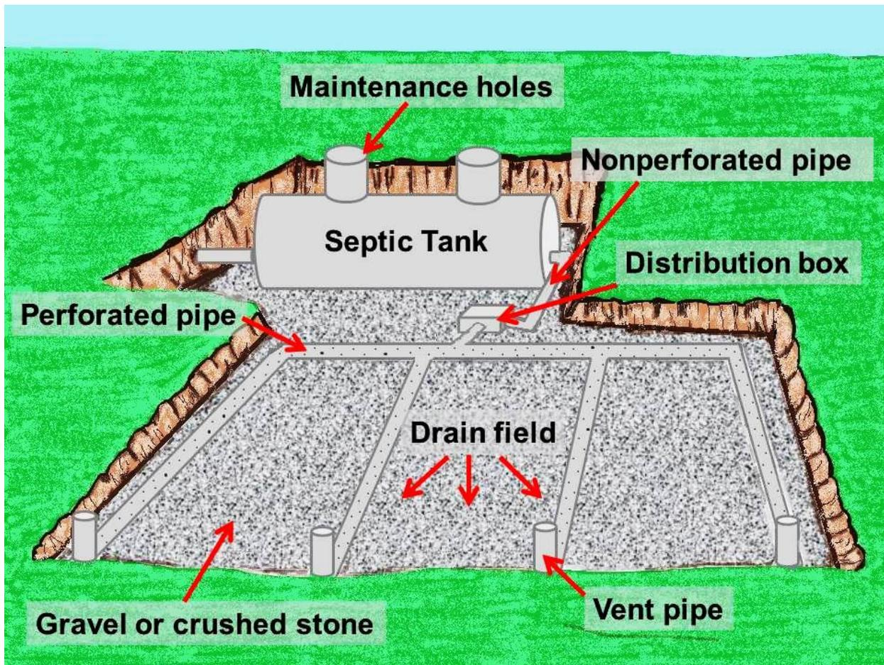
Effluent flows directly from your household plumbing into a watertight, underground, two compartment septic tank. Solid waste settles into a sludge layer on the bottom and fats float to the top of the first compartment. Between these two scum layers is a zone of clarified liquid effluent which is internally piped to the second compartment of the septic tank for additional settling.
