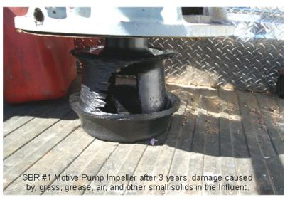
Various damage from undesirable materials in the sewer system. Bottom, heavy grease from not being regularly pumped. Photograph credit John Bougham.
