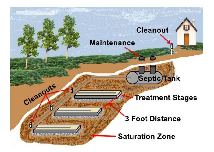
A 10-foot separation is used for most applications. Also, if both ends of the drain cannot be extended to the ground surface, the upslope end should be extended some distance along the surface contour beyond the end of the SWIS.
