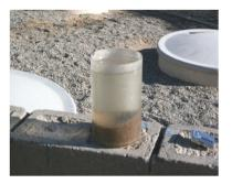
This growth form is important as these flocs degrade BOD and settle at the end of the process, producing a low TSS effluent.
