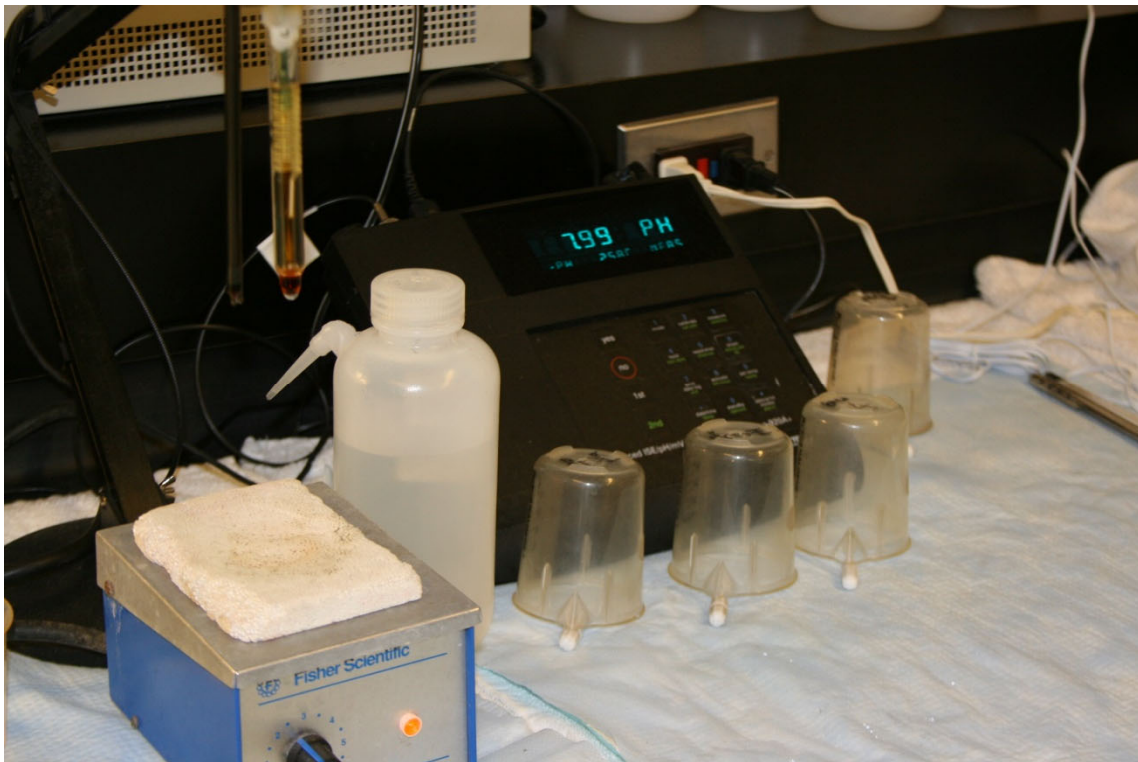
Electronic pH probe, a WWT tool you will use every day.
