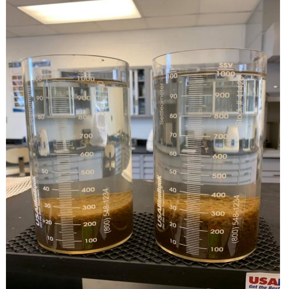
Well-settled mixed liquor with a clear supernatant
