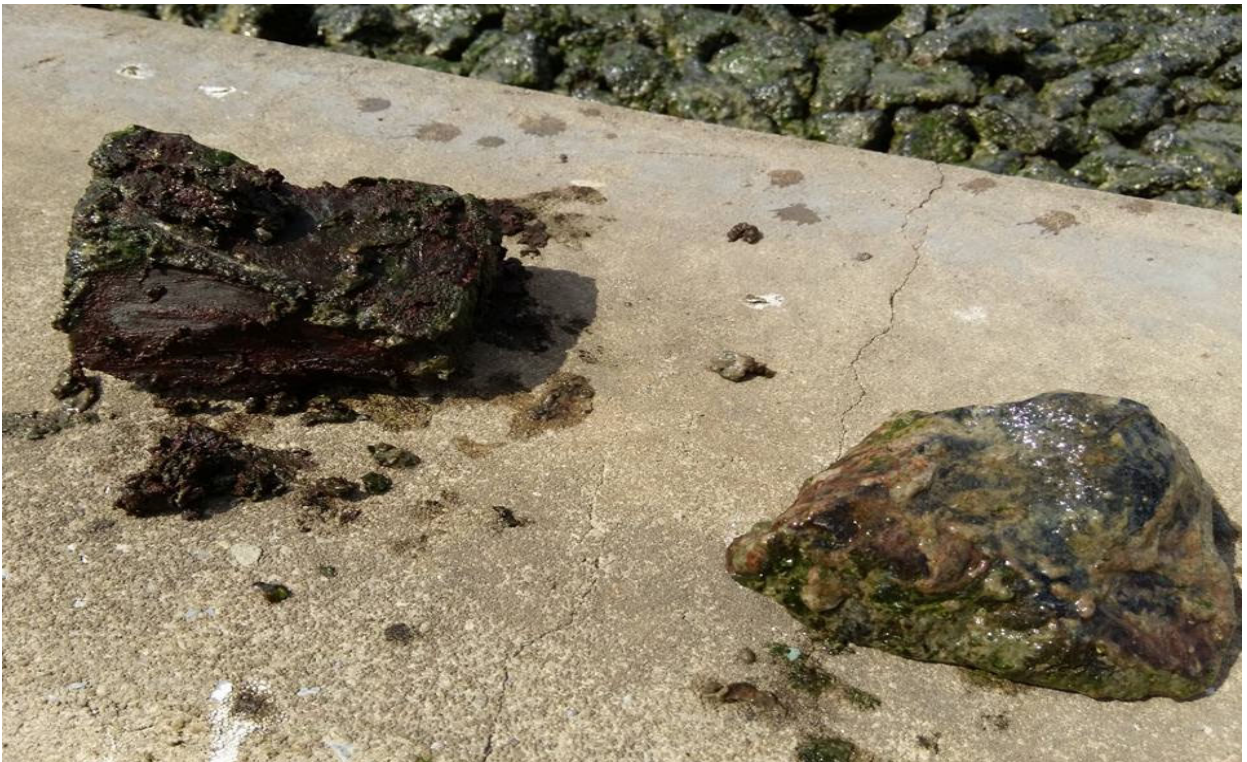
Fixed-film trickling filters. The left filter discoloration is due to sloughing. The photo below is the actual material off that filter.
