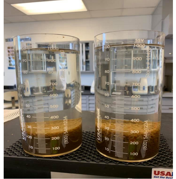
Well-settled mixed liquor with a clear supernatant
