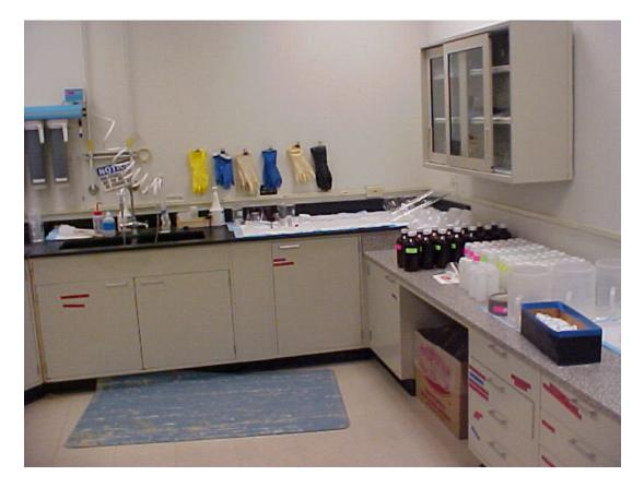
Notice the anti-slip mat and the several different types of gloves necessary to handle the different chemicals that could be present. Notice how each bottle and drawer is clearly marked.
