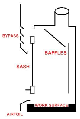
**3.5 Bypass** - grill opening above face of hood that helps to maintain a constant face velocity independent of the sash position. When the sash is lowered air flows in through the bypass and the hood face. When the sash is raised it blocks the bypass.
