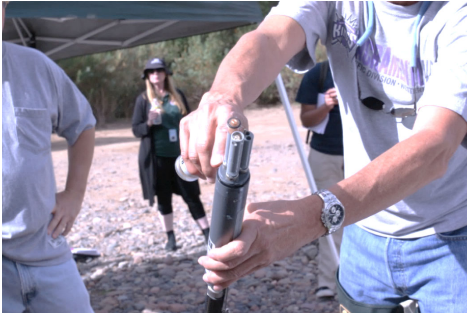
Top Photo: This multi probe device measures dissolved oxygen (DO), pH, conductivity and total dissolved solids (TDS), the device requires calibration for each parameter.
