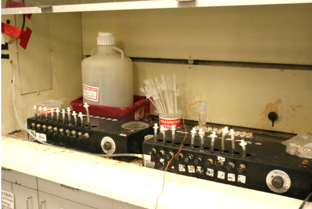
Top Photo: This area is used for Fecal coliform which the most common dilution is prepared by transferring 11 ml of sample to 99 ml of sterile phosphate dilution water using a sterile serological pipet.
