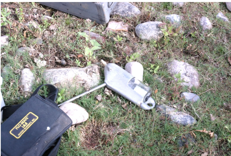
Bottom Photo: Collection of isokinetic, depth-integrated samples is done using either an equal-width-increment (EWI) or equal-discharge-increment (EDI) sampling method. The methods typically result in a composite sample that represents the streamflow-weighted concentrations of the stream cross section being sampled. That sample is poured into the bottles that resemble old fashion milk bottles.
