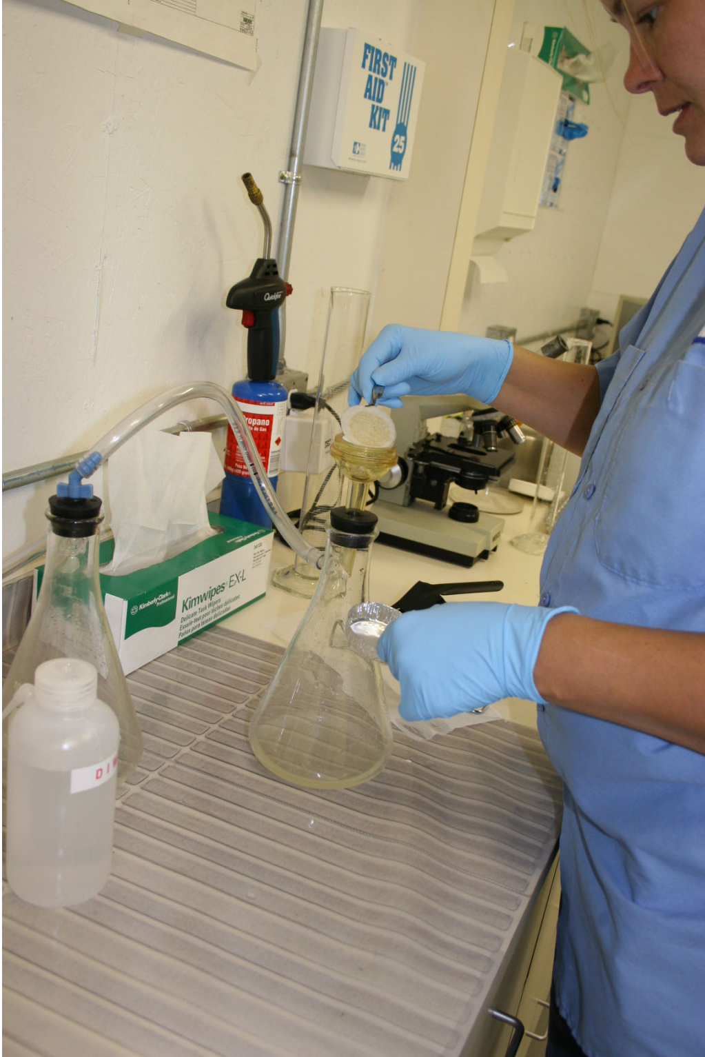
Lab tech removing filter for TSS analysis.
