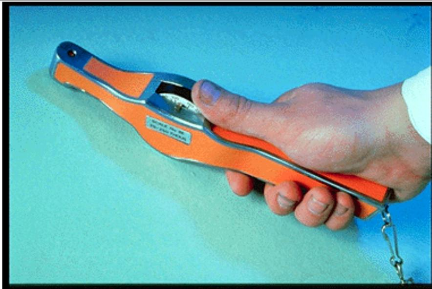
Testing a recently applied tank lining for uniformity in thickness.
