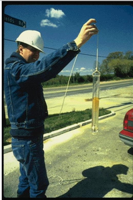
Collecting a sample of gasoline from a monitoring well using a clear bailer.
