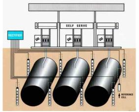
(iv) and the integrity of the tank is ensured using one of the following methods:(i) The tank is internally inspected and assessed to ensure that the tank is structurally sound and free of corrosion holes prior to installing the Cathodic protection system; or
