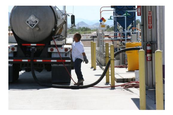
This photograph shows a delivery of Sulfuric Acid. The delivery driver is wearing only work gloves. He is clearly in violation of the proper PPE. The Hazard Communication Standard requires employees to understand chemical hazards, labels, and SDSs and to use them on the job. Before starting jobs involving possible exposure to hazardous substances, employees must read SDSs to know what they're working with and procedures for safe handling.
