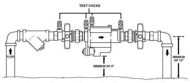
REDUCED PRESSURE PRINCIPLE BACKFLOW PREVENTER DIAGRAM
