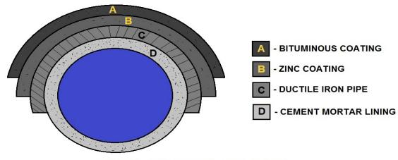
**DUCTILE PIPE DETAIL**
