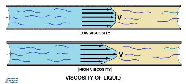
**Viscosity of liquids** in chemistry is the resistance to flow exhibited by fluids (liquids or gases) like glycerol, ester, oils, water, alcohol, ether. The flow of some liquids is slower than the others due to this property.
