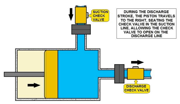
PISTON TYPE -POSITIVE DISPLACEMENT PUMP
