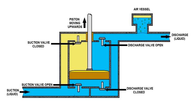
POSITIVE DISPLACEMENT PUMP RECIPROCATING PISTON TYPE
