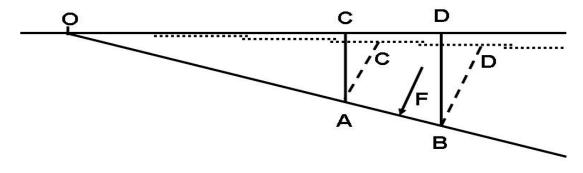
THRUST ON A PLANE DIAGRAM
