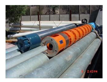
Large Diameter Submersible Pump, Motor, and Column Pipe
