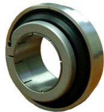
The type of material used for the seal faces will depend upon the service of the pump. Most water service pumps use a carbon material for one of the seal faces and ceramic (tungsten carbide) for the other. When the seals wear out, they are simply replaced.
