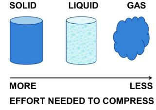
compress. Many shock absorbers in cars compress liquids in tubes.
