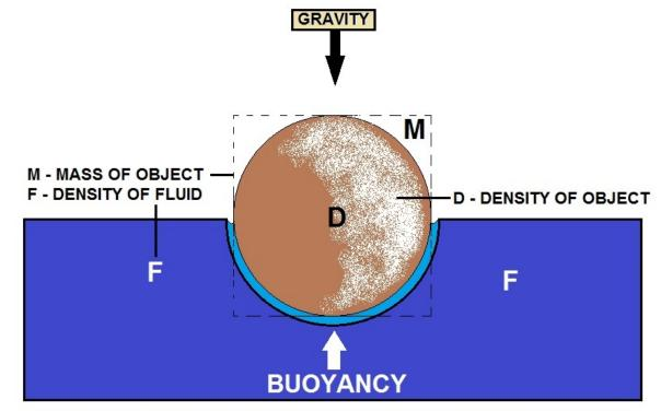
BASICS THAT IMPACT HOW BUOYANCY WORKS
