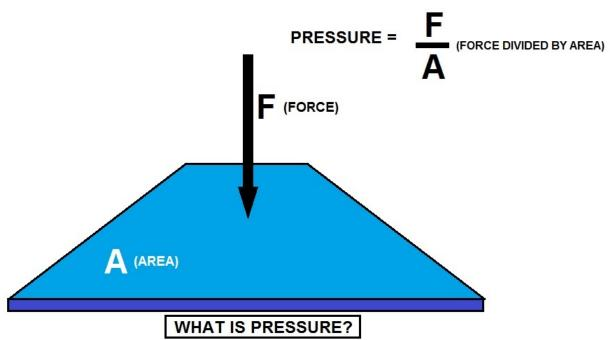
PRESSURE IS THE AMOUNT OF FORCE ACTING ON A SPECIFIC AREA AND IS EQUAL TO THE FORCE DIVIDED BY THE AREA
