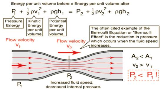
A special form of the Euler's equation derived along a fluid flow streamline is often called the **Bernoulli Equation.**
