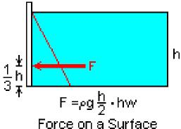
integral of dM' = pgxy dA, the moment about some vertical line in the plane of the surface. If there happens to be a pressure on the free surface of the water, then the forces due to this pressure can be evaluated separately and added to this result. We must add a force equal to the area of the surface times the additional pressure, and a moment equal to the product of this force and the distance to the centroid of the surface.
