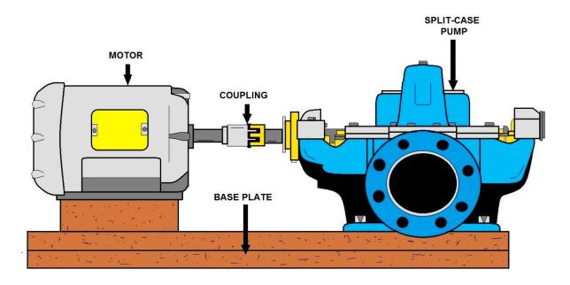
FLEXIBLE COUPLED PUMP AND MOTOR
