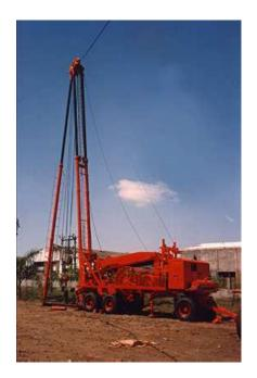
Typical Cable Tool Rig
