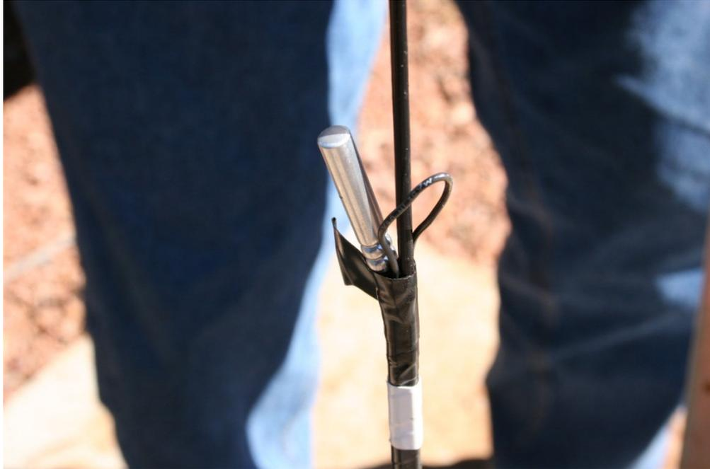
Blasting cap on the explosive cord. Below, some of the debris from inside the well casing following the explosion. After talking to this man, I found out that after 9-11, he had to increase his fees because of the ATF and new rules concerning explosives. Be prepared to pay through the nose for this treatment process. Consider this fee the price of admission for having adequate water to supply your customer's demands.
