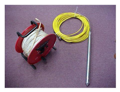
Groundwater Transducer (pH, Temp. chemical detection, and D.O.) and depth probe. These tools are used to find the depth and pH of well water.
