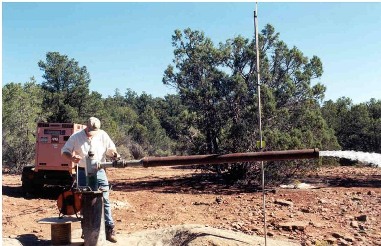
Well pumping test being conducted in photograph above. (Notice the portable electric generator for powering the pump. The Hydrogeologist is using a depth probe to measure the drop in the static water level.)
