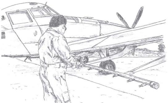
PILOT DOING PRE-FLIGHT CHECKS ON NOZZLES
