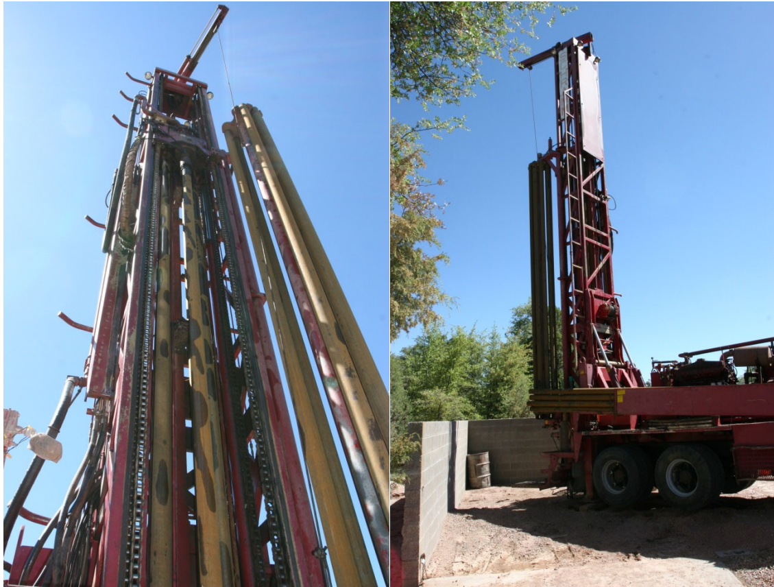
Top, drill rigging mast. Below, drilling rods on carousel and rack, notice copper pipe thread coating which prevents thread lock during high torque.
