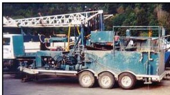
Small Self-Contained Mud System
