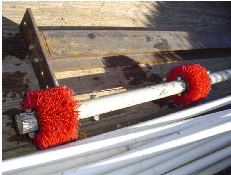
This type of brush is used to dislodge debris inside well casing.
