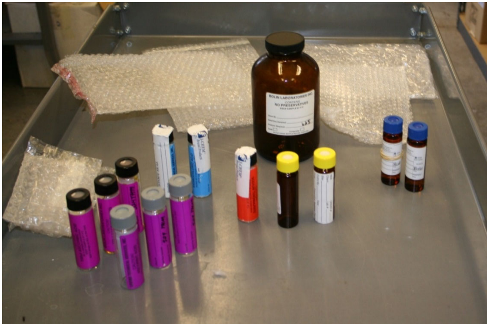
Various water sample bottles and chain-of-custody form.
